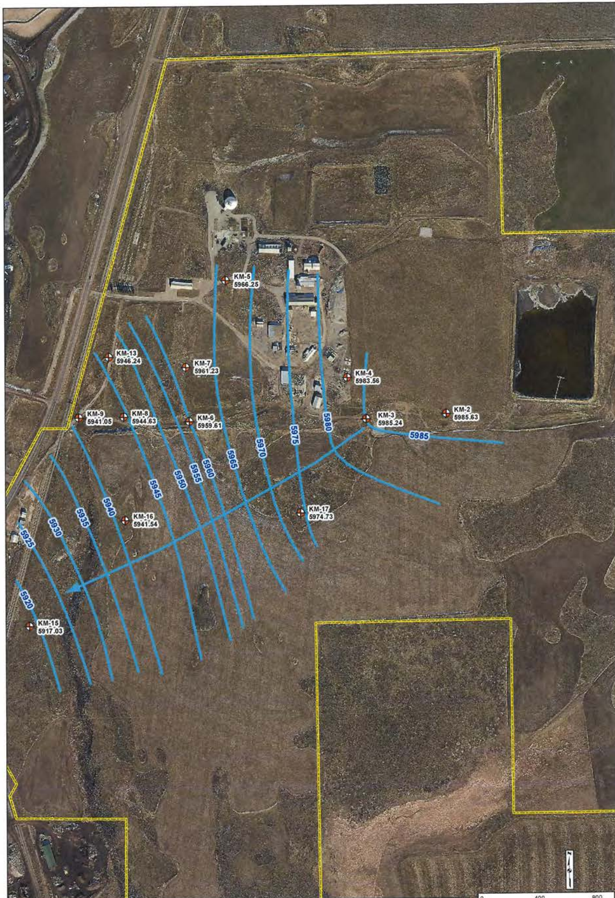
FIGURE 5 SHALLOW GROUNDWATER POTENTIOMETRIC SURFACE - SEPTEMBER, 2015 GROUNDWATER / SURFACE WATER REPORT, 2015 DATA
