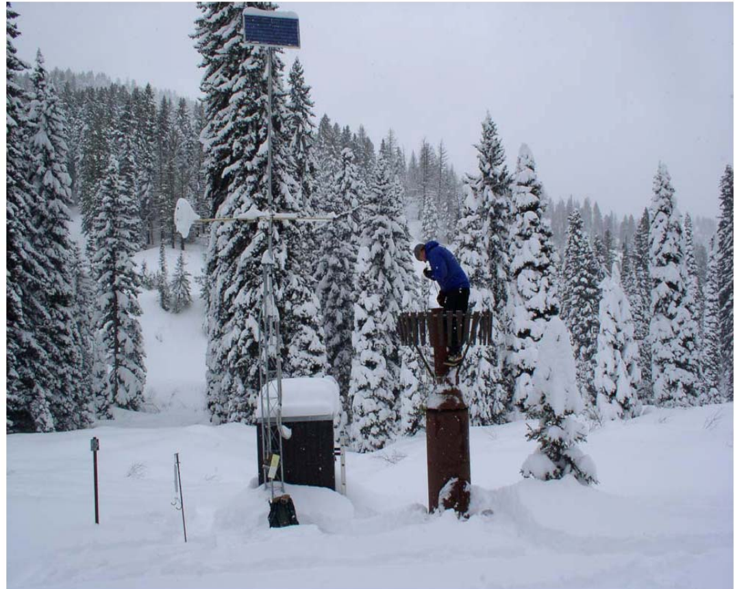
NRCS hydrologist, Jeff Anderson, uses large weight on a rope to knock a snow plug into propylene glycol antifreeze solution inside the SNOTEL precipitation gage at Mores Creek Summit, Idaho, February 28, 2007.
