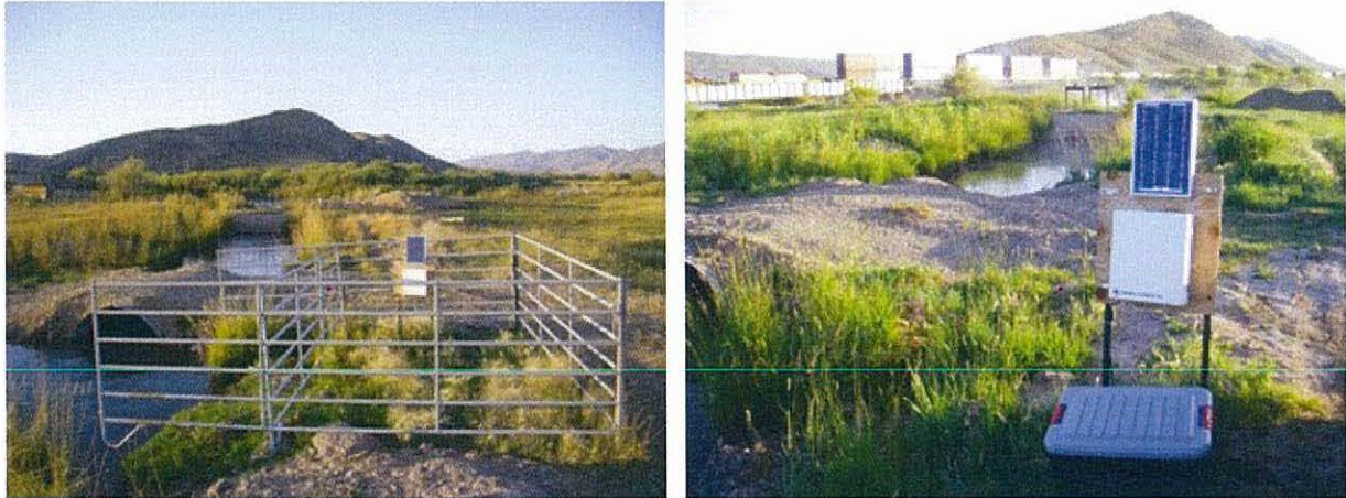
Figure 6 – Installation of DFM systems on Nuffer Diversion. Right hand picture depicts the Unidata DFM deployment, enclosure and power supply are located behind fencing for protection from cattle, squash pipe is located in stream adjacent to DFM system, and the diversion works can be seen in background approximately 100 feet upstream of the squash pipe. The left hand picture is a close up of the Unidata DFM system, note the weather proof container at the base of the fence posts where the MACE DFM system was temporarily housed.
