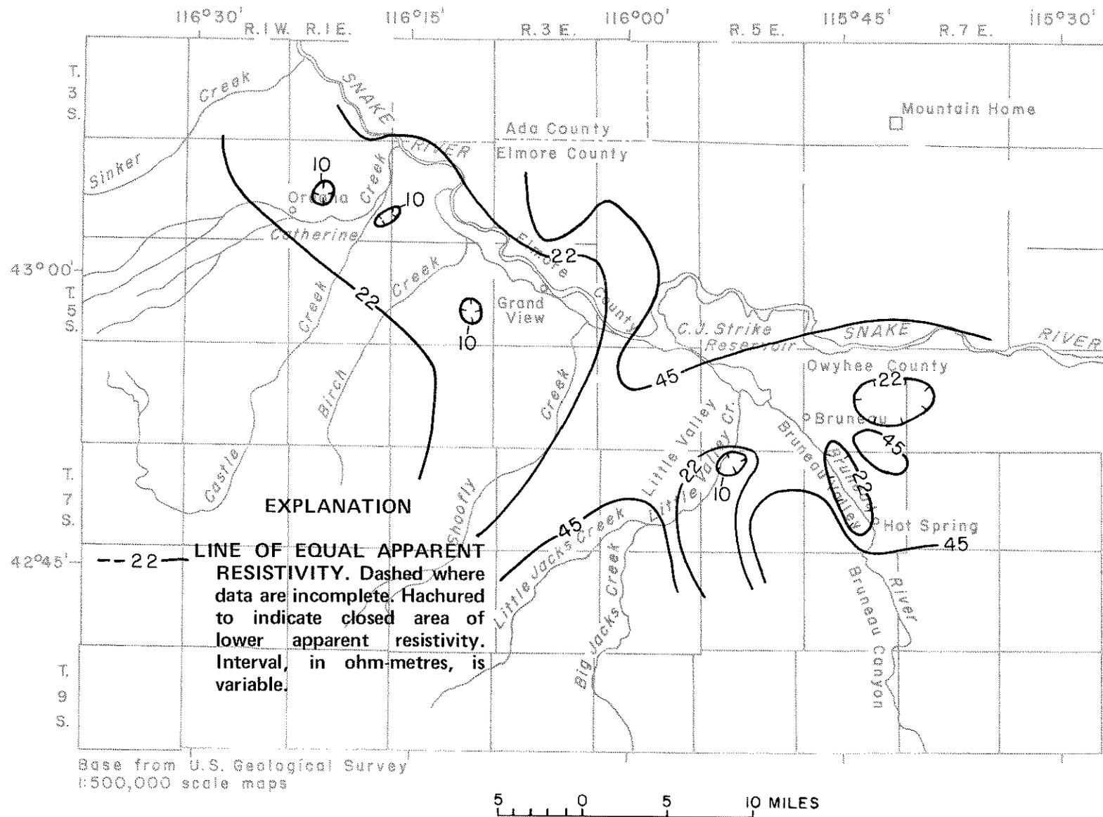
FIGURE 24. Apparent resistivity map at 18,600 hertz.
