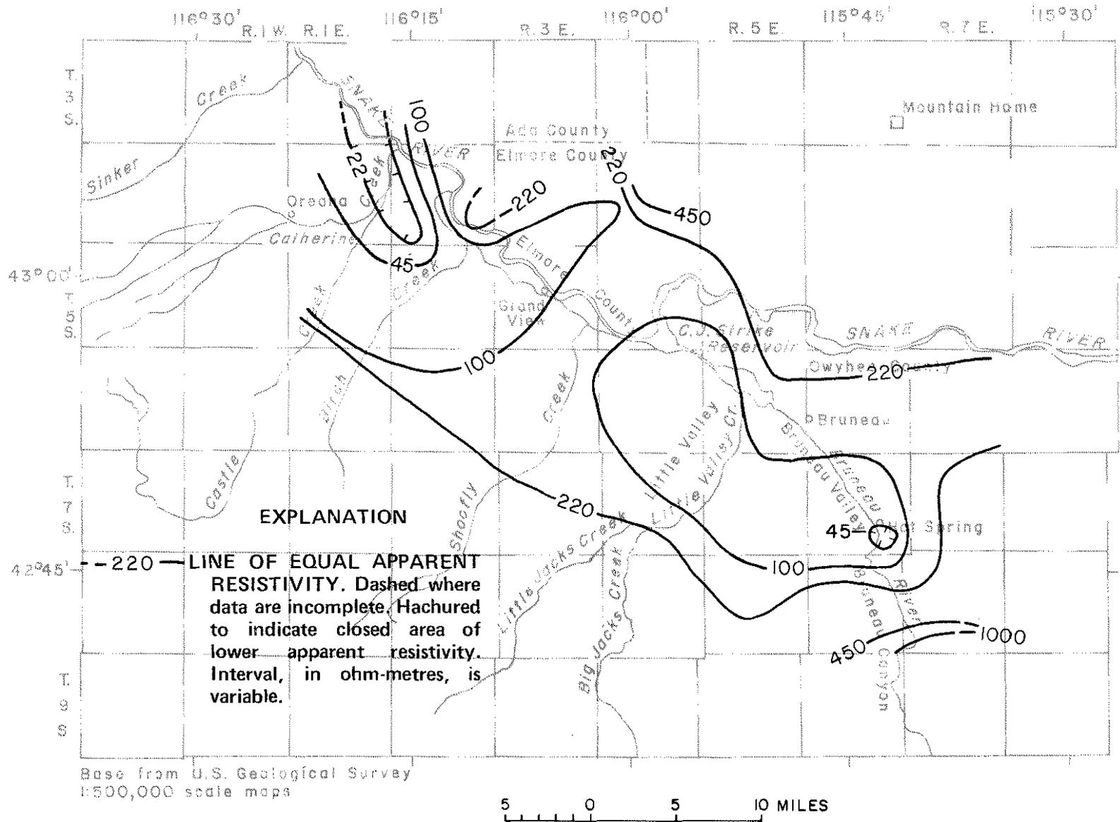
FIGURE 22. Apparent resistivity map at 700 hertz.
