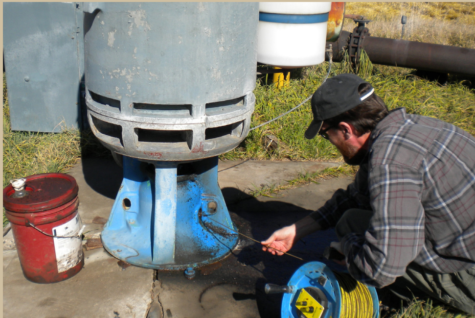
IDWR hydrology staff routinely measure water levels in approximately 550 ESPA wells two times a year. (IDWR photo)
