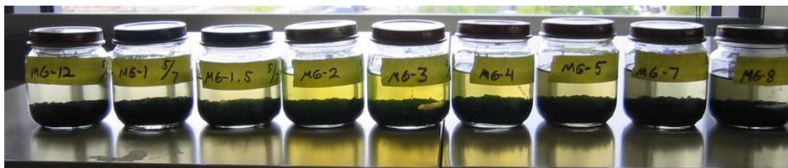
Figure 12. Charcoal soaking in eluting solution from Fluorescein Test #1 visually showing dye in MG-1.5 through 5.
