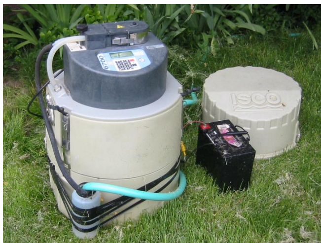
Figure 17. ISCO auto sampler deployed at Riddle well #26 programmed to collect 500 mL samples every 12 hours from a constant flow through container.
