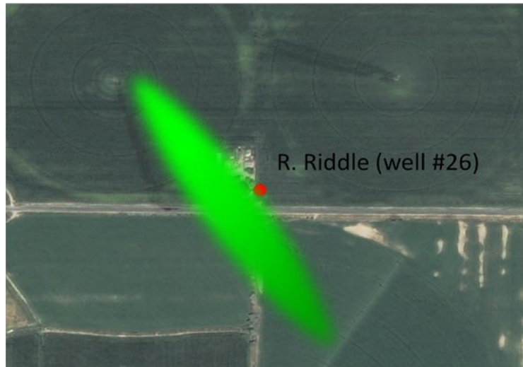
Figure 19. Conceptual dye cloud showing how Riddle well #26 may have intersected the edge of the cloud thereby effecting the timing and magnitude of concentration measured at this location.
