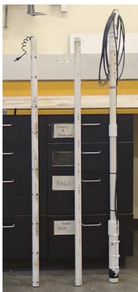
Figure 2: The first probe on the left has a wire connection, which requires a USB connection to a computer or table, the one in the center is the new wireless version and the download wireless bar on the right.
