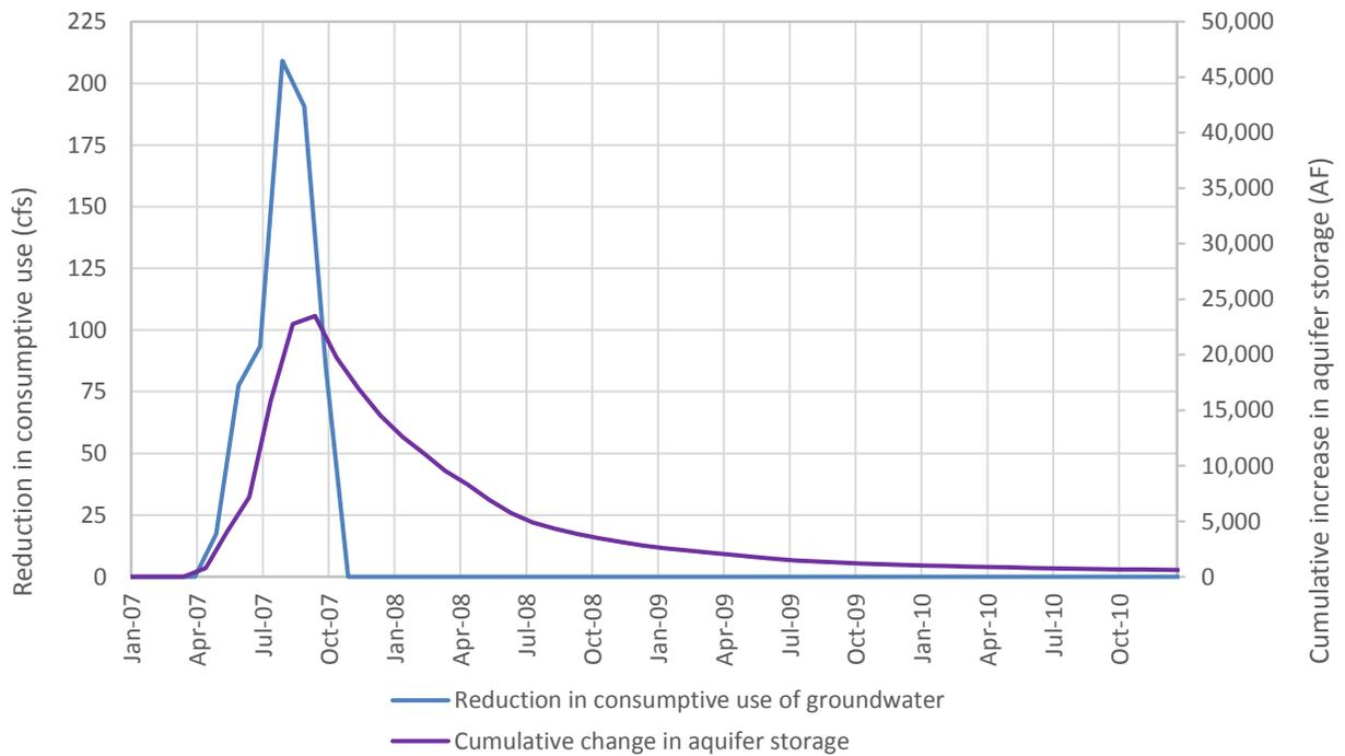
Figure 10. Change in aquifer storage resulting from simulated curtailment of non-exempt groundwater irrigation (2007)
