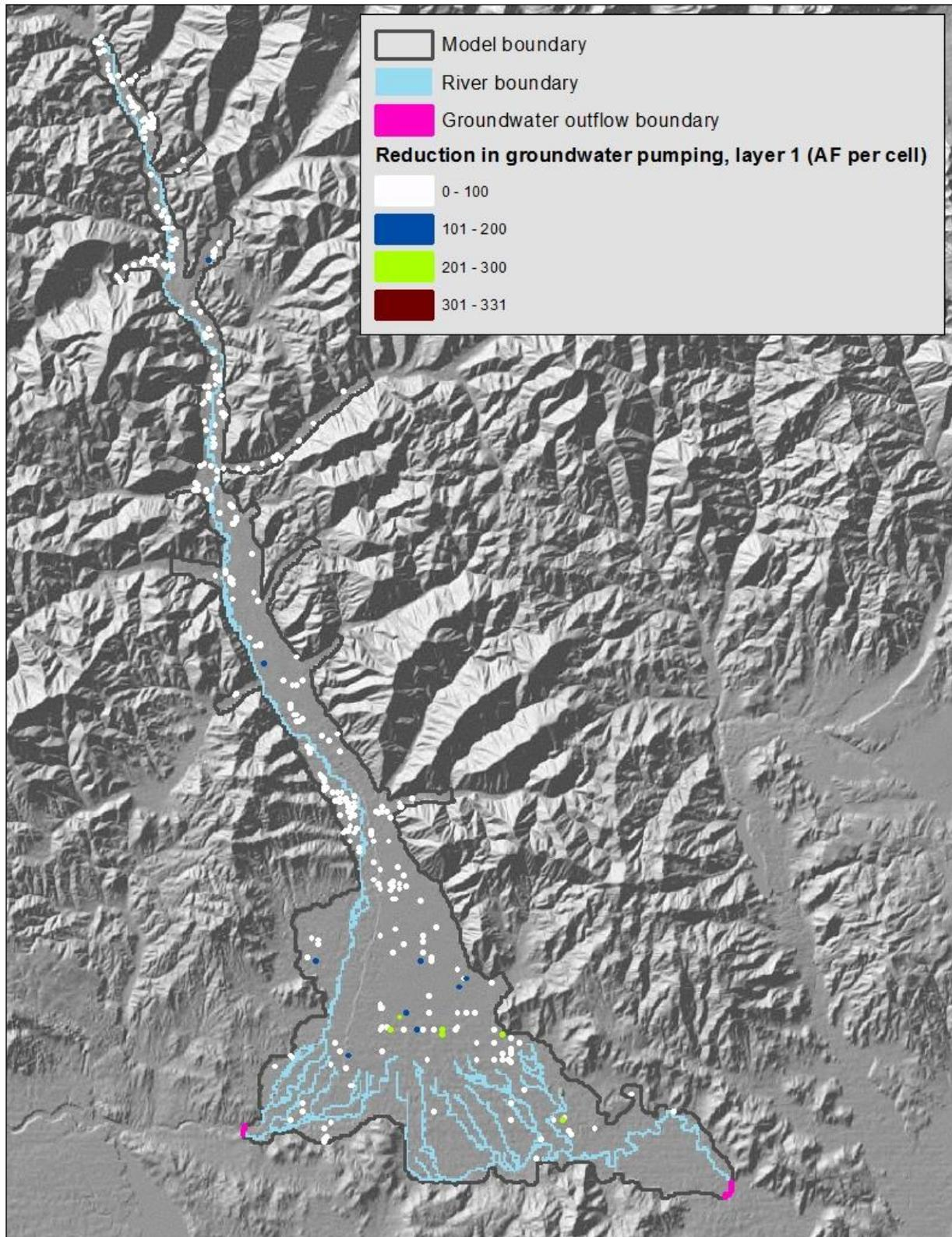
Figure 1. Spatial distribution of simulated reduction in groundwater pumping within model layer 1 (monthly stress from August 2007 shown as an example)
