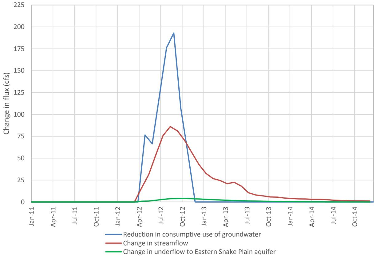
Figure 13. Hydrologic responses to simulated curtailment of non-exempt groundwater irrigation (2012)
