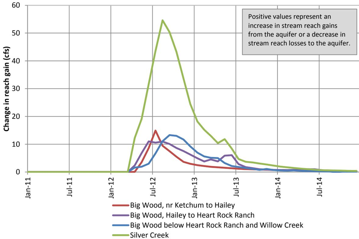
Figure 15. Predicted increase in streamflow in response to curtailment of non-exempt groundwater irrigation (2012)
