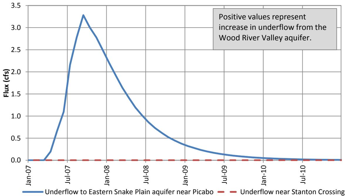
Figure 12. Predicted increase in groundwater outflow in response to curtailment of non-exempt groundwater irrigation (2007)
