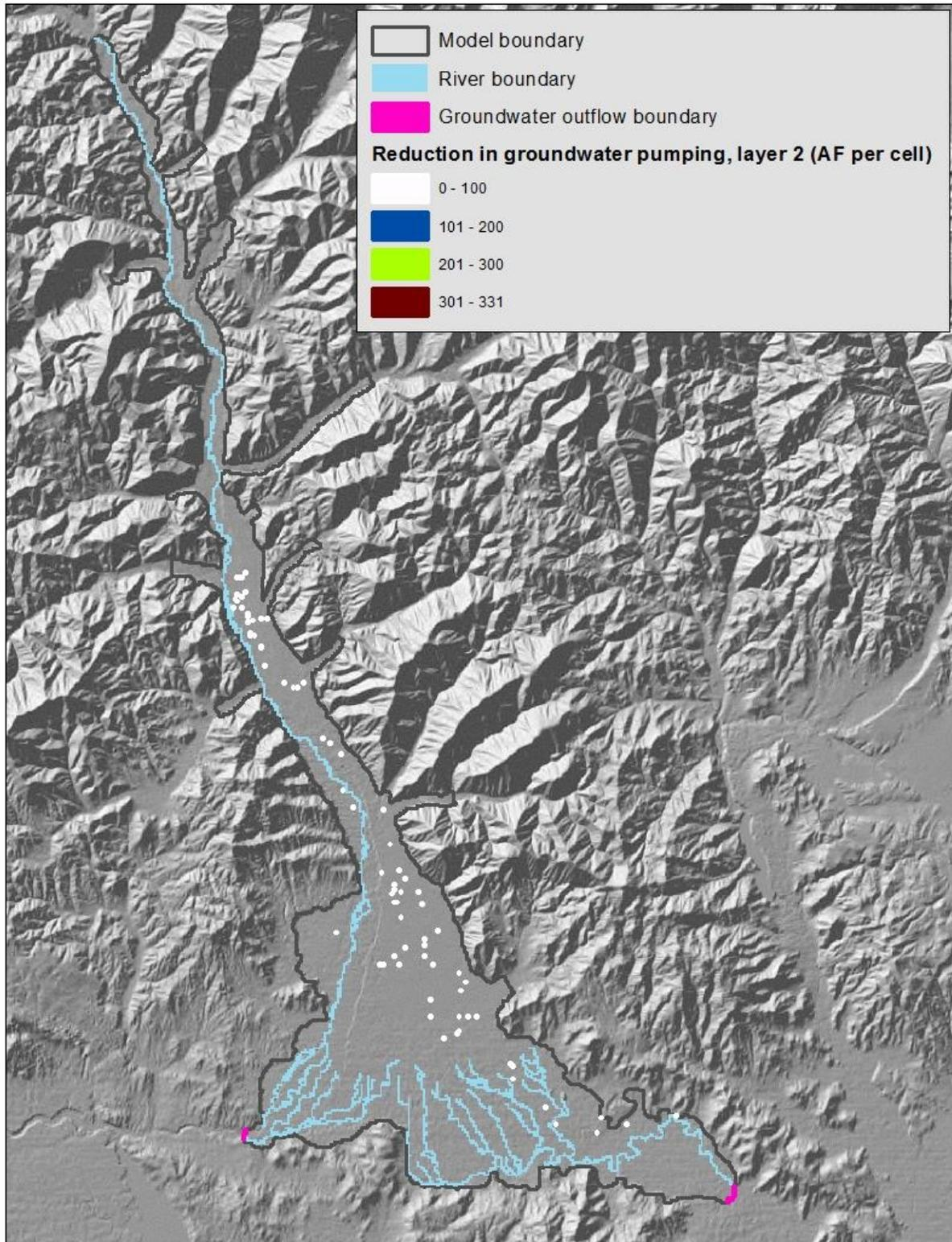
Figure 2. Spatial distribution of simulated reduction in groundwater pumping within model layer 2 (monthly stress from August 2007 shown as an example)
