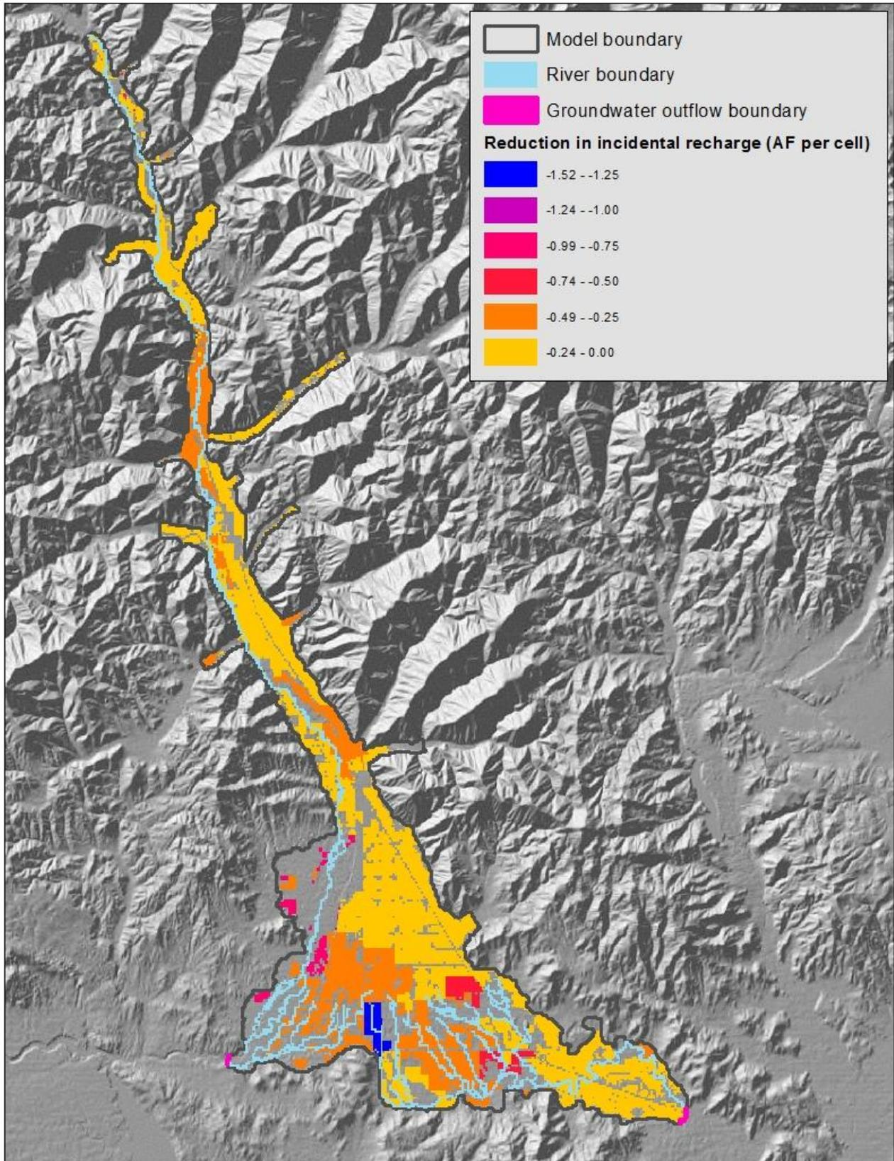
Figure 4. Spatial distribution of simulated reduction in incidental recharge within model layer 1 (monthly stress from August 2007 shown as an example)
