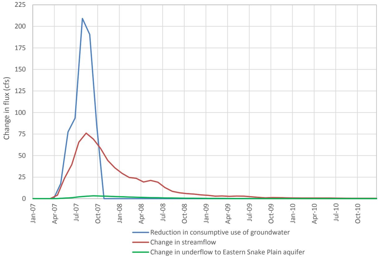
Figure 9. Hydrologic responses to simulated curtailment of non-exempt groundwater irrigation (2007)
