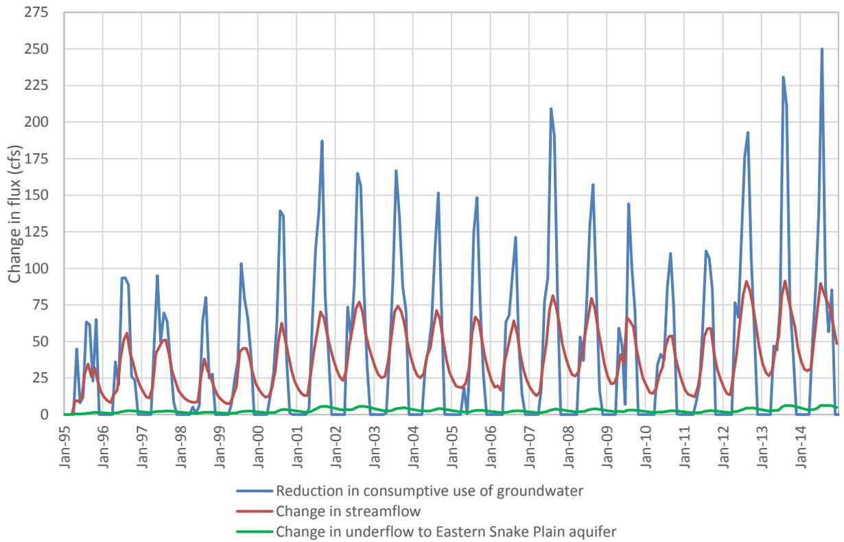
Figure 5. Hydrologic response to simulated curtailment of non-exempt groundwater irrigation (1995-2014)
