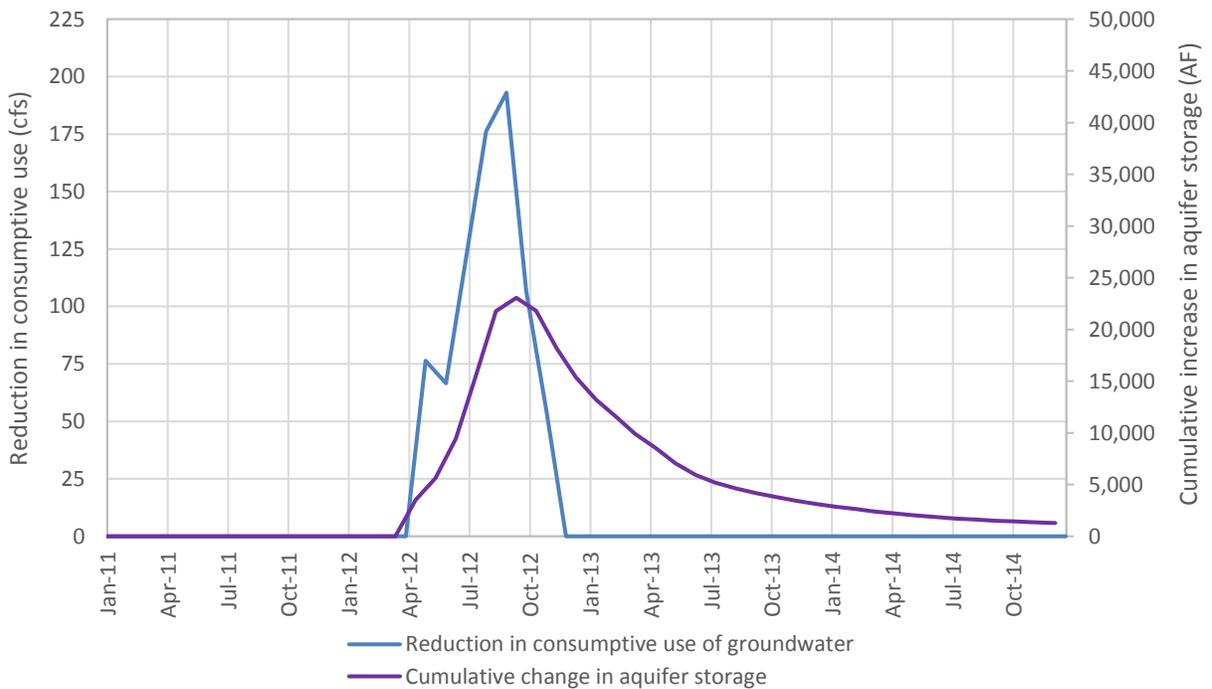
Figure 14. Change in aquifer storage resulting from simulated curtailment of non-exempt groundwater irrigation (2012)
