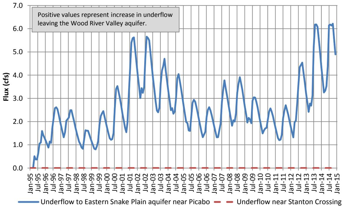
Figure 8. Predicted increase in groundwater outflow in response to curtailment of non-exempt groundwater irrigation (1995-2014)
