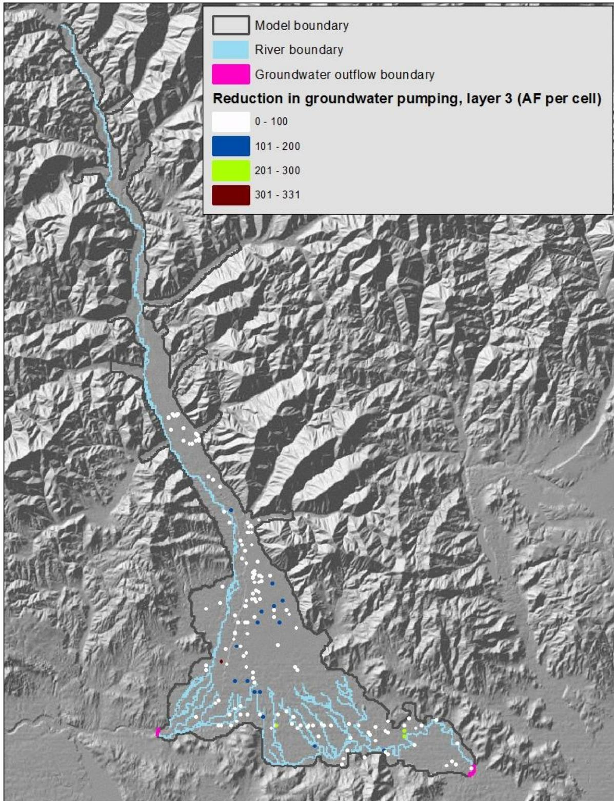
Figure 3. Spatial distribution of simulated reduction in groundwater pumping within model layer 3 (monthly stress from August 2007 shown as an example)
