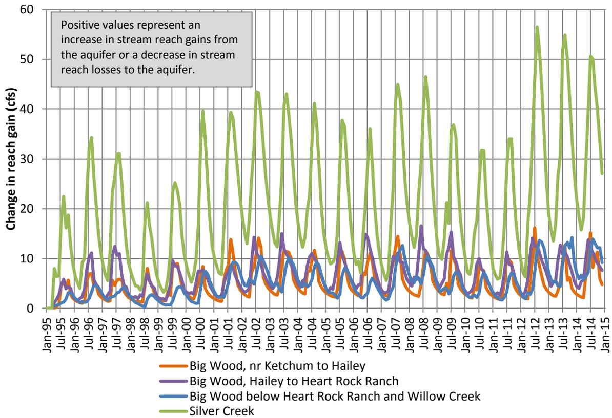
Figure 7. Predicted increase in streamflow in response to curtailment of non-exempt groundwater irrigation (1995-2014)
