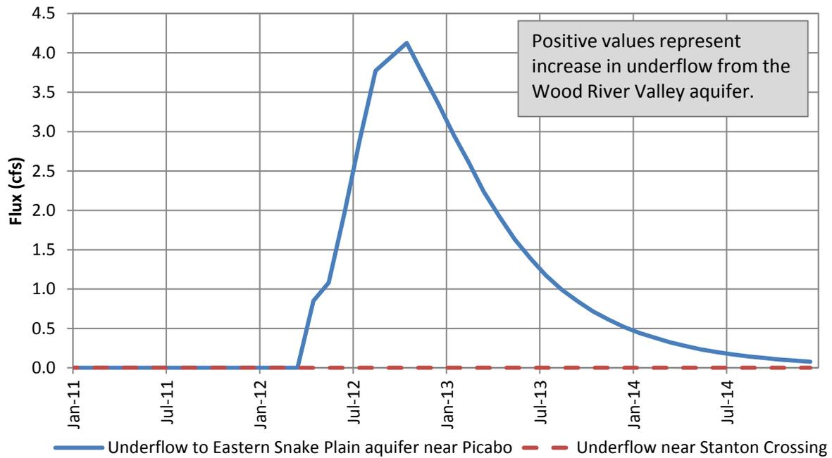
Figure 16. Predicted increase in groundwater outflow in response to curtailment of non-exempt groundwater irrigation (2012)
