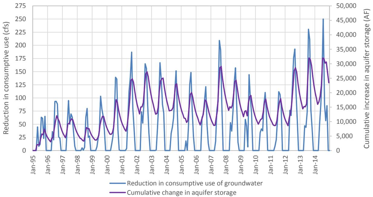
Figure 6. Change in aquifer storage resulting from simulated curtailment of non-exempt groundwater irrigation (1995-2014)
