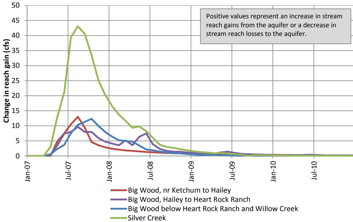
Figure 11. Predicted increase in streamflow in response to curtailment of non-exempt groundwater irrigation (2007)
