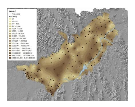
PEST adjusts pilot point value and interpolates values for cells between pilot points
