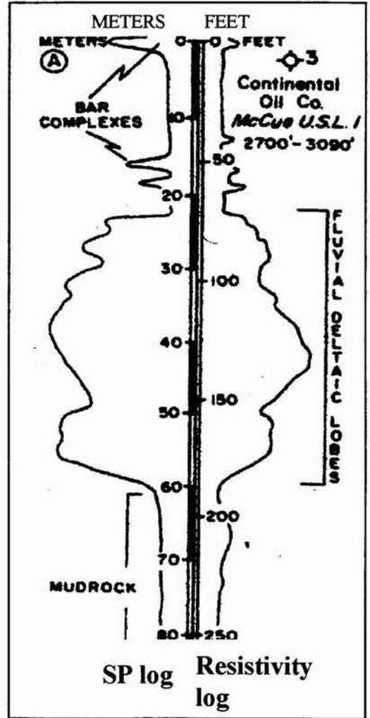
Figure 6. SP and resistivity log of lacustrine prodelta mudrock overlain by delta sand lobes, overlain by a mouth-bar complex: Ridge-Basin, California (from Link and Osborne, 1978).
