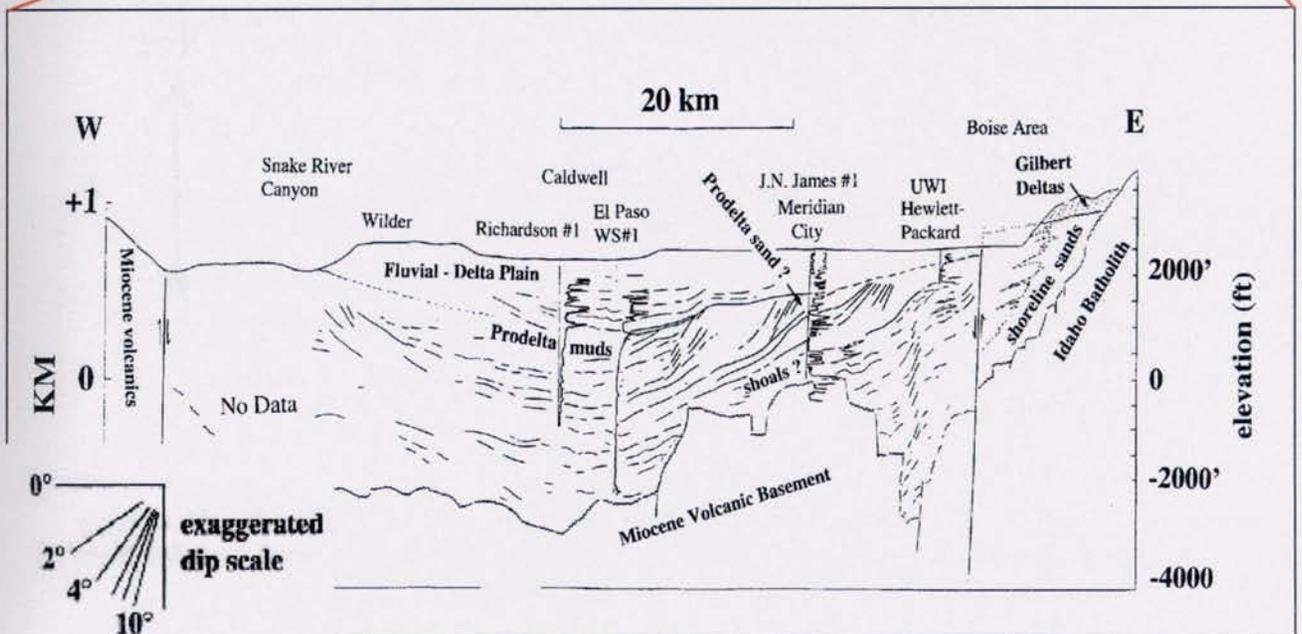
Figure 2. Interpreted cross-section from seismic lines across the western Snake River Plain, showing the geometry of strata that reflect seismic waves within lake and stream deposits and the resistivity response of borehole geophysical logs of deep wells. Drawn from petroleum industry seismic reflections lines which were focused on the deeper strata and did not image the strata shallower than 700 ft depth (i.e., the main cold-water aquifer section).
