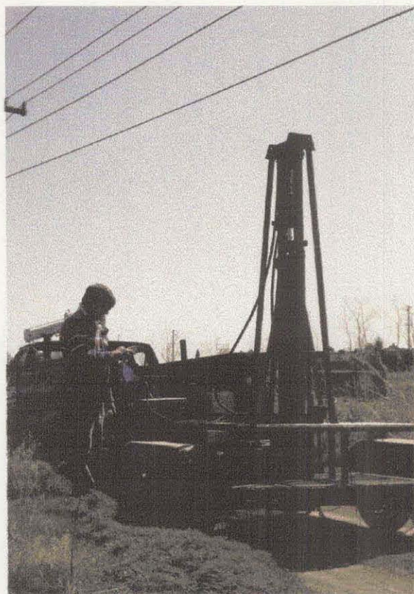
FIGURE 4. (A) The trailer-mounted seismic source used for the seismic reflection project. (B) Annotated shot gather from site NT1 along the downtown railroad spur near Orchard Road. Processing includes f-k and 40-150 Hz spectral whitening filters and air wave mute and shows the data quality of the raw field records.
