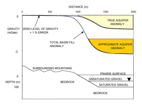
Figure 8. Geology section and the gravity response over a typical aquifer boundary. The gravity effect of the aquifer extends to about one kilometer outside the aquifer boundary.
