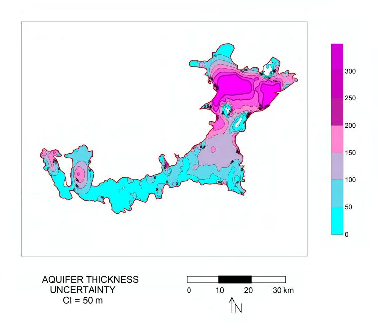
Figure 13. The uncertainty in aquifer thickness due to lack of gravity stations on the periphery of the aquifer boundary.
