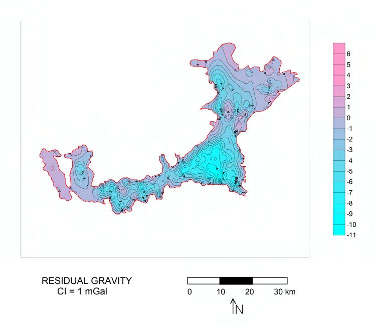
Figure 10. The residual gravity representing the original Bouguer gravity with the effects of the regional trend removed.
