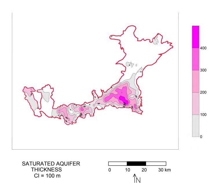
Figure 11. Isopach of the aquifer based on residual gravity.
