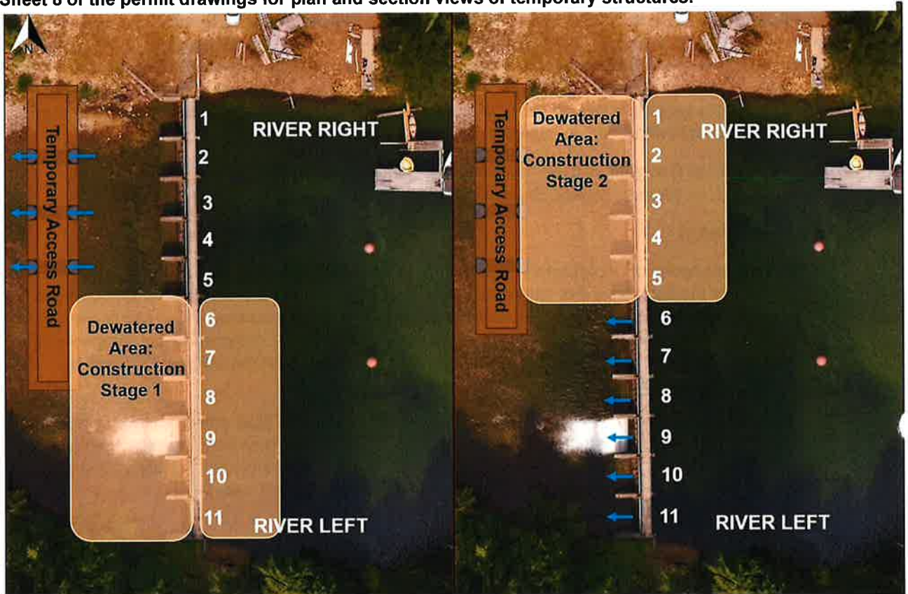
Figure 2: Outlet Structure construction sequence schematic; Stage 1 (south) and Stage 2 (north). See Sheet 8 of the permit drawings for plan and section views of temporary structures.
