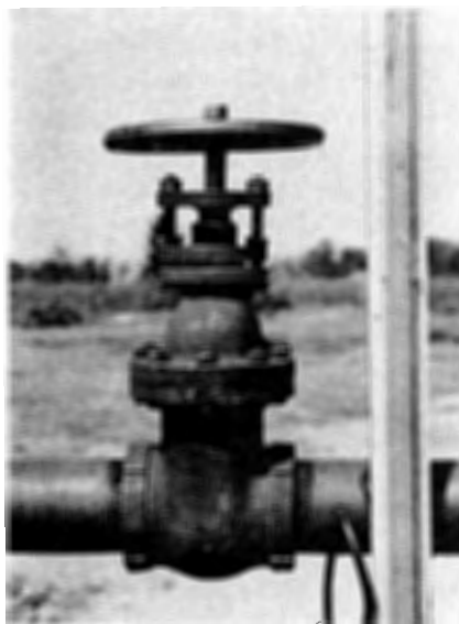
Figure 19 Four inch gate control valve used to maintain a constant head on the discharge orifice.
