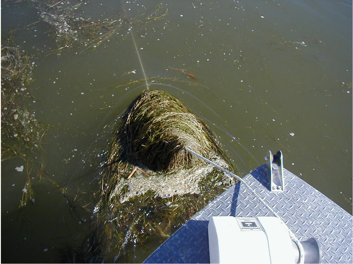
Macrophyte build-up on sampling equipment at Indian Cove. Cable had been in the water for 4 minutes. Photo: Idaho Power Company.
