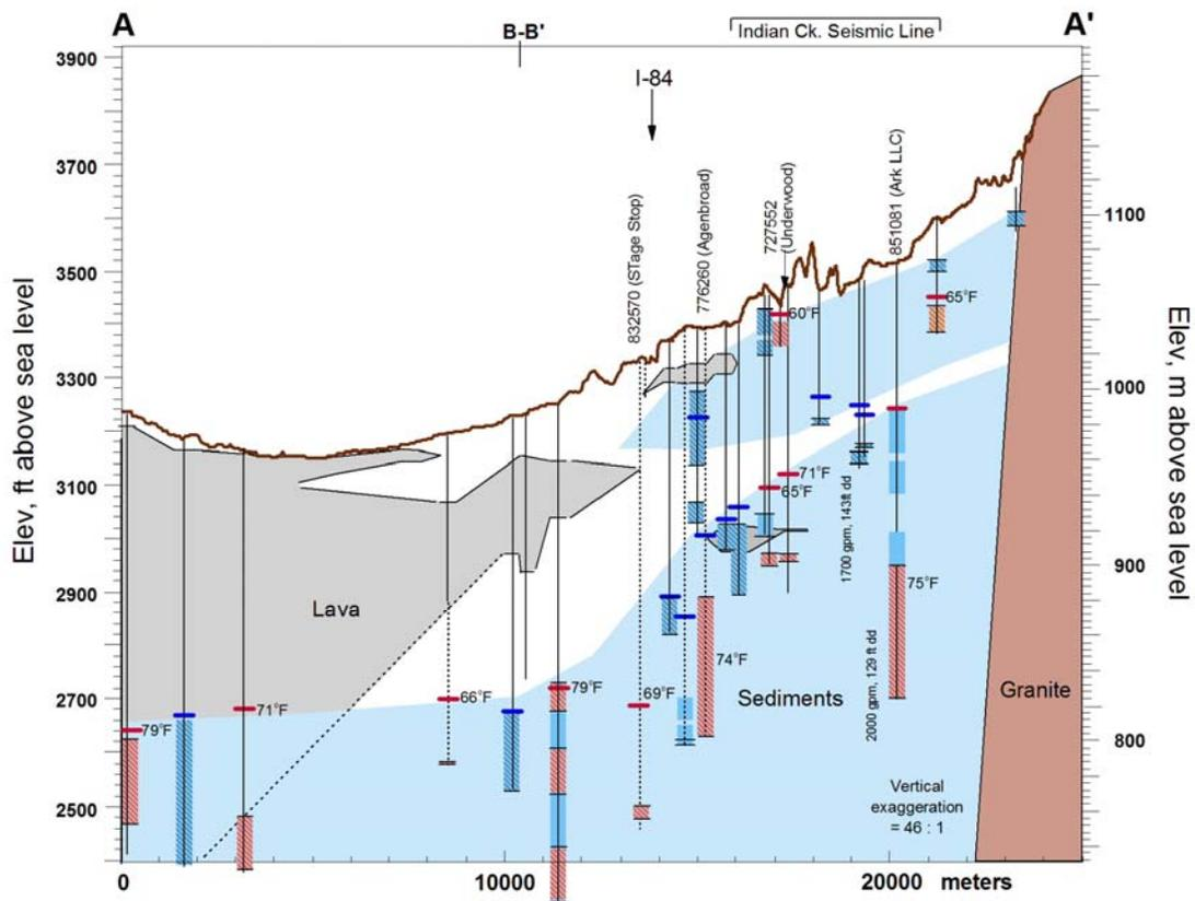
Figure 9 - A simplified interpretation of possible aquifer geometry along section A-A' based on reported static water levels as well as the locations of reported water-bearing zones.
