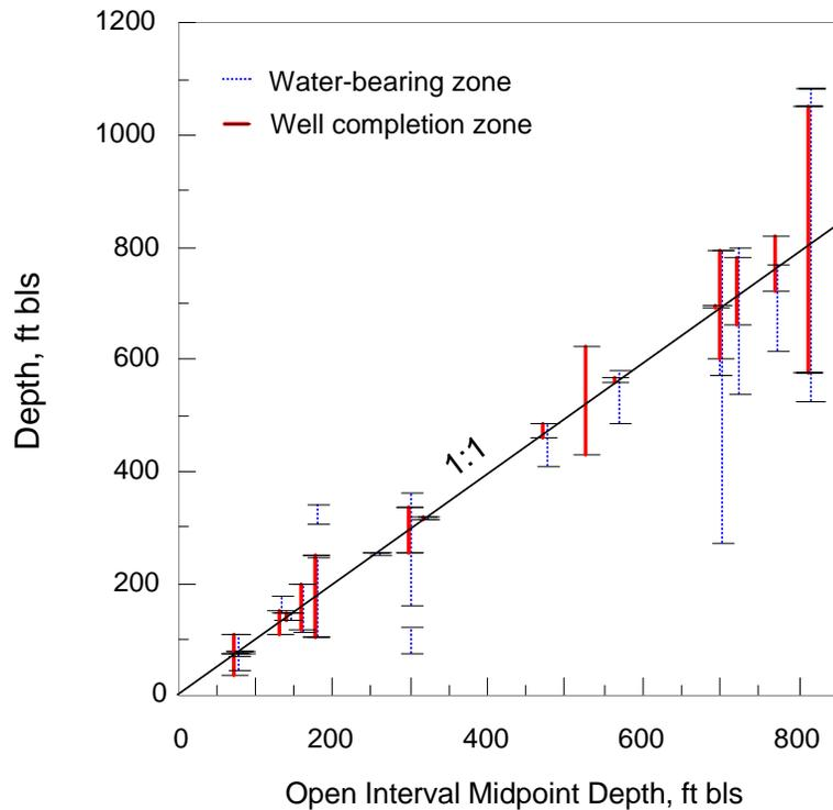
Figure 7 - Summary of depths at which drillers reported encountering water in wells along section A-A' and depth intervals over which the wells were eventually completed.
