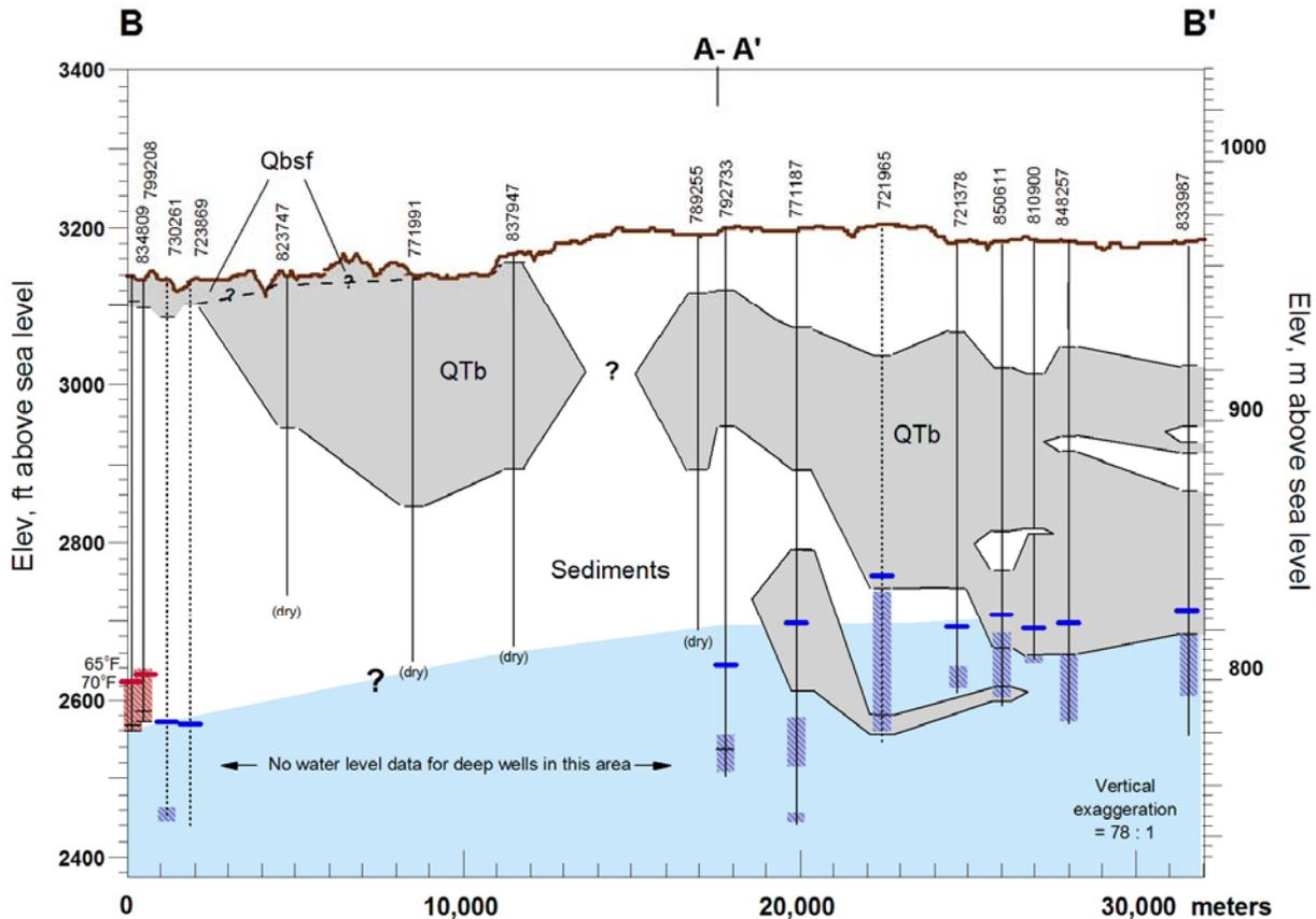
Figure 10 - Possible aquifer geometry based on depths of reported water-bearing zones and static water levels along section B-B'.
