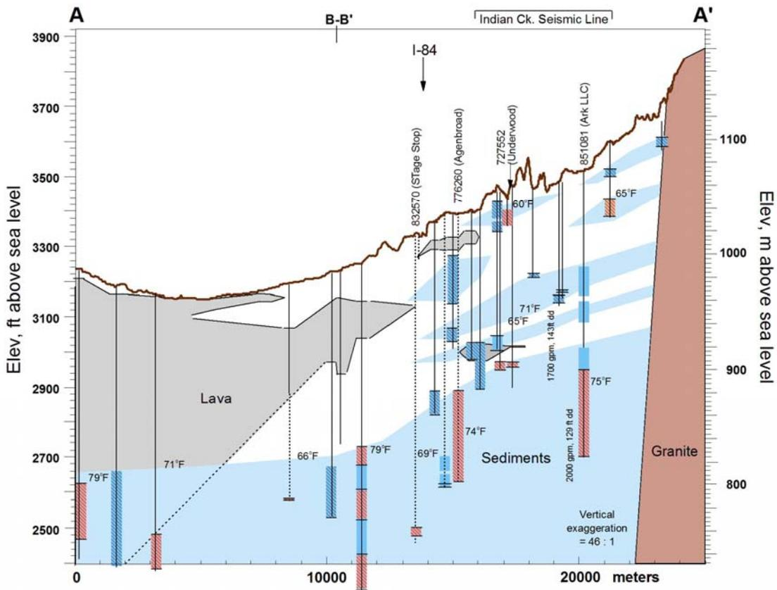
Figure 8 - One of many possible interpretation of aquifer geometry along section A-A' based solely on the locations of reported water-bearing zones.
