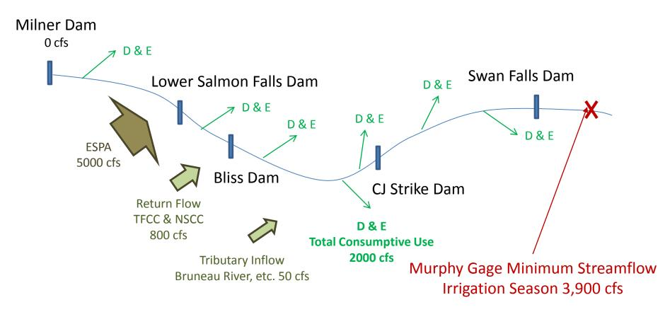
$5000 \text{ cfs} + 800 \text{ cfs} + 50 \text{ cfs} - 2000 \text{ cfs} = 3,850 \text{ cfs} = Actual Flow Condition}$  Shortfall = 100 ac-ft
