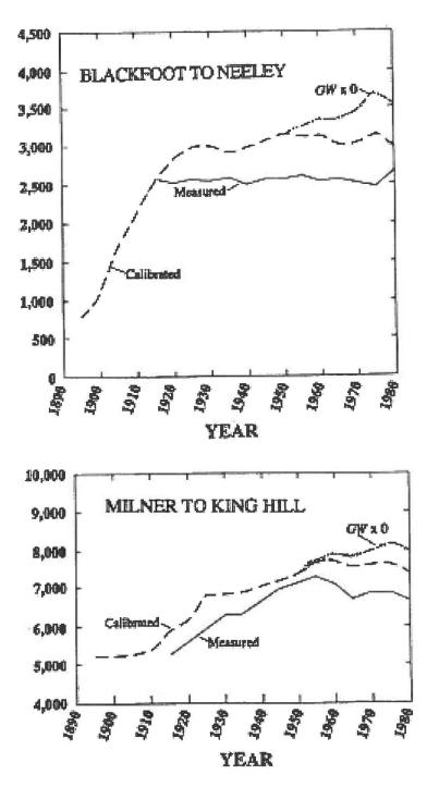
Figure 3. USGS RASA Transient Simulations - Reach Gains in Cfs
