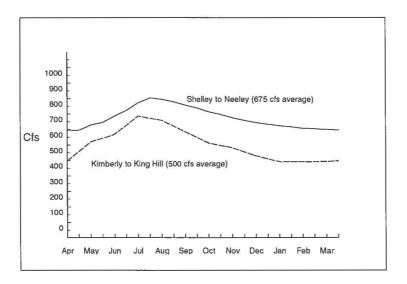
Figure 2. Changes in Reach Gains Resulting from Ground Water Pumping over ESPA after 25 years.
