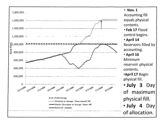
Any empty space in the reservoir at the time of maximum physical fill is the result of the inaccurate prediction of how much storage water must be dumped out of the reservoir to create empty reservoirs for flood control.
