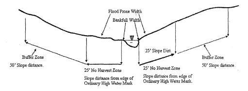
SINGLE CONFINED CHANNEL: Bank full flow is contained within a single channel and the flood prone width in less than four times the bank full channel width
