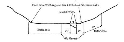
SINGLE UNCONFINED CHANNEL: Bank full flow is contained within a single channel and the flood prone width is greater than four times the bank full channel width.
