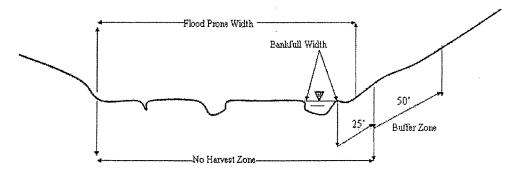
MULTIPLE UNCONFINED CHANNELS: Bankfull flow occupies multiple (braided) channels and the flood prone width is greater than four times the bankfull channel width.
