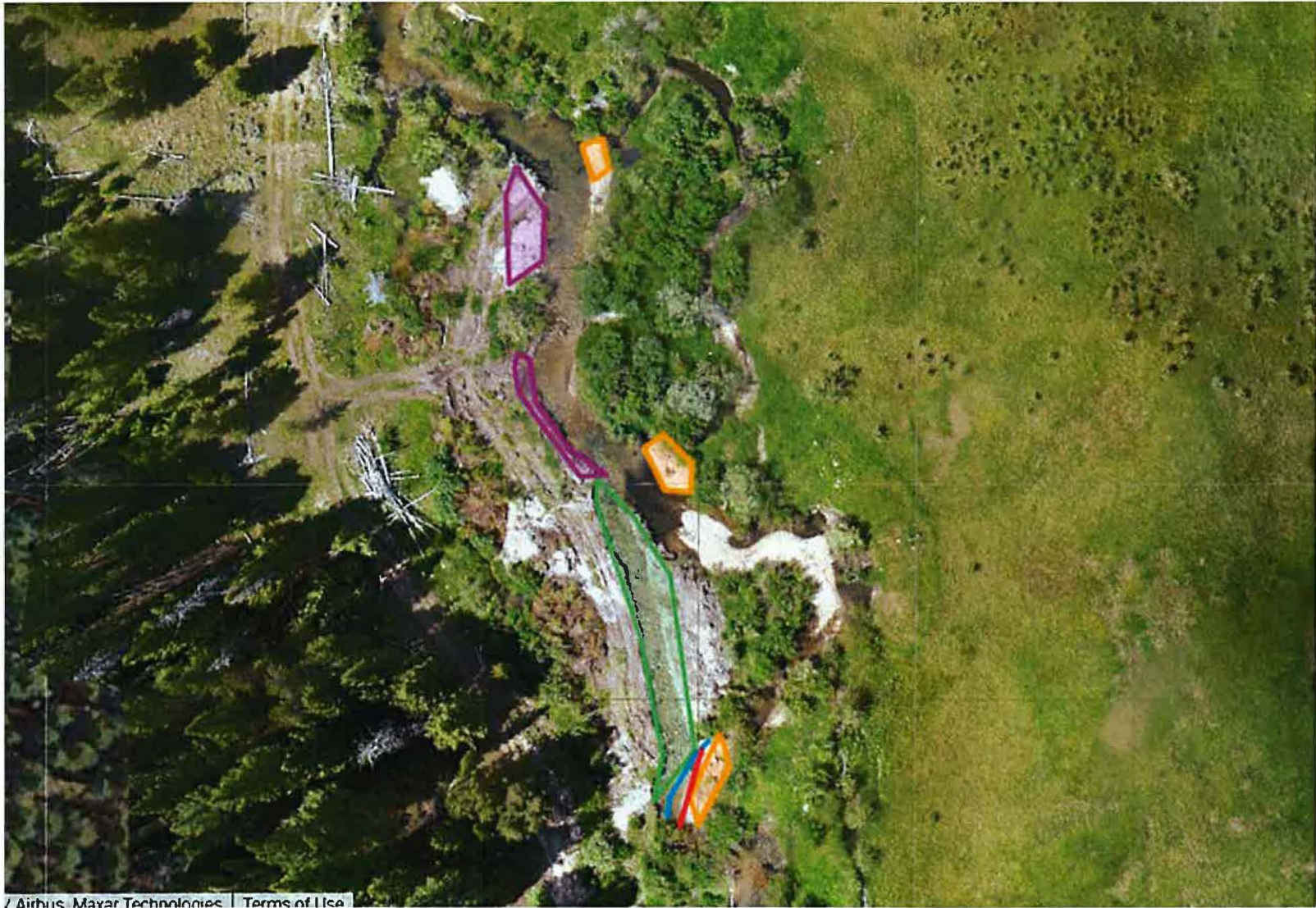
Figure 5. Site 5 - Multiple ditch/channel intercepts over short distance. Extensive left bank reconstruction likely required.
