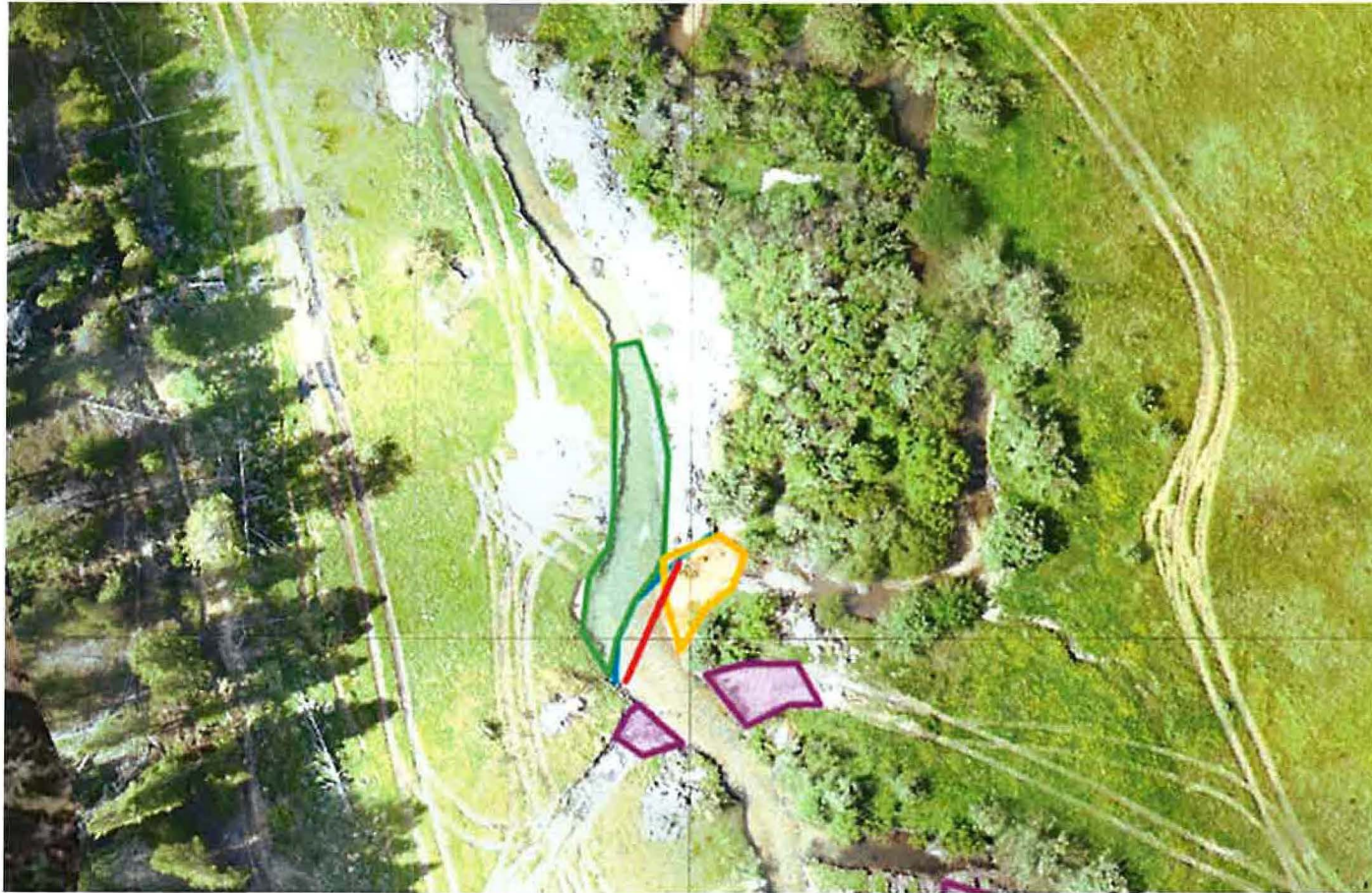
Figure 2. Site 2 - Second ditch/channel diversion point. Portion of ditch appears to be constructed in historic channel meander (overlaps w/ford location).
