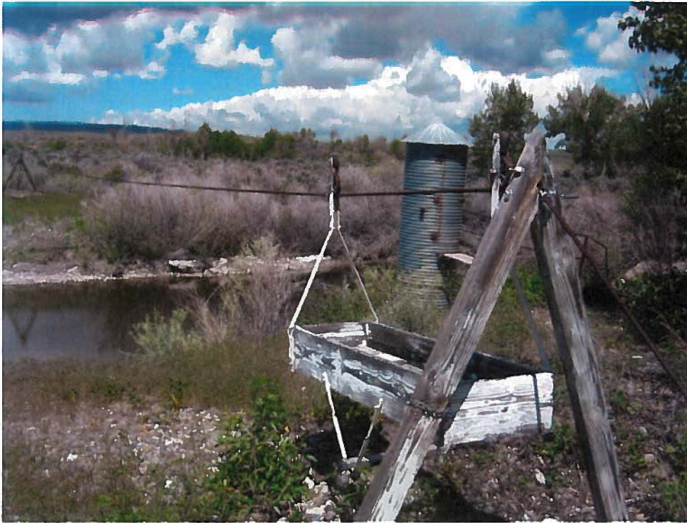
10. Big Wood River Gage Station #5 located in river below Richfield Canal spill gates; cable care in foreground and stilling well behind it.
