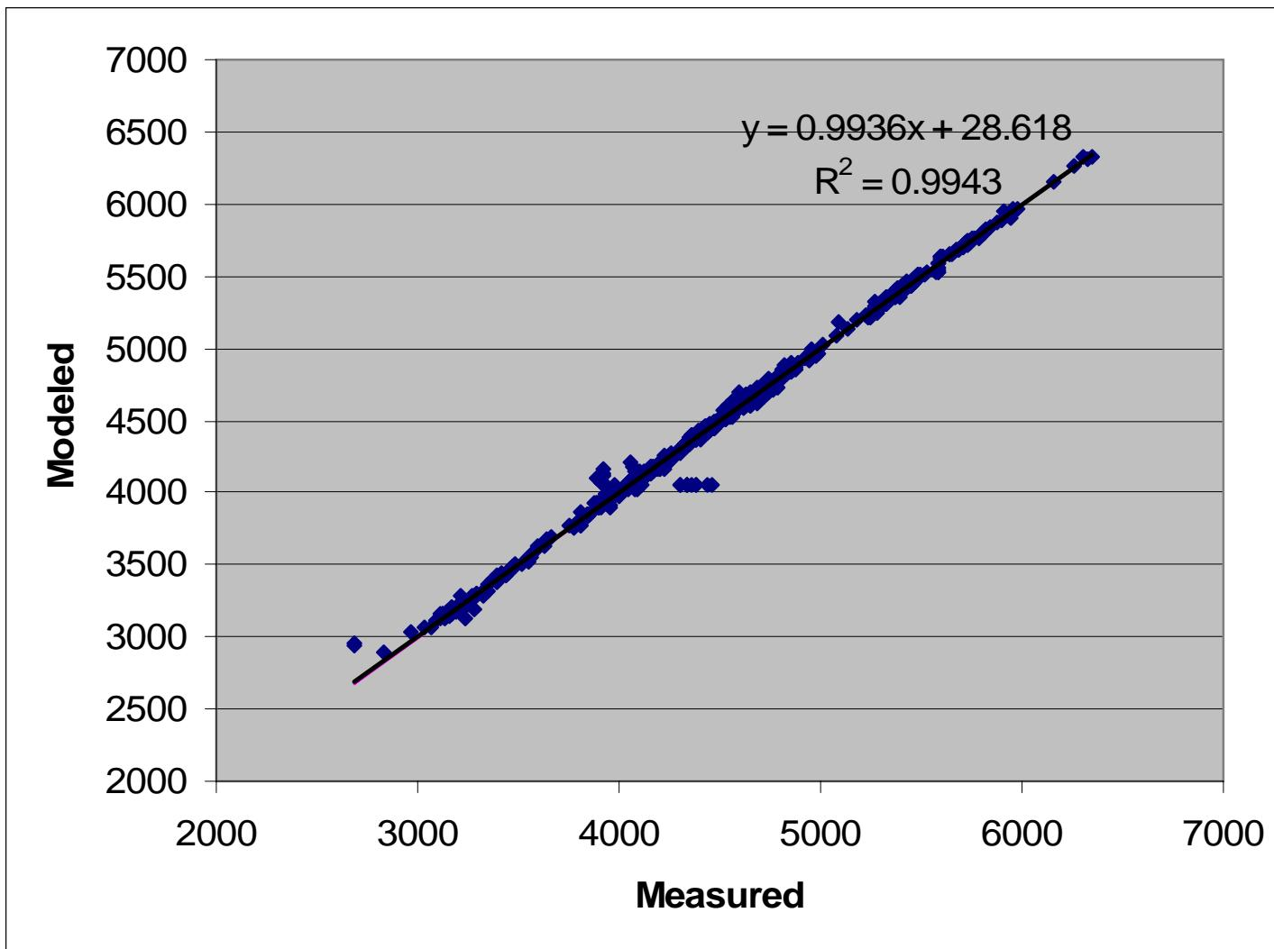
Figure 58. Scatter plot of model-predicted versus observed steady aquifer water levels (ft).
