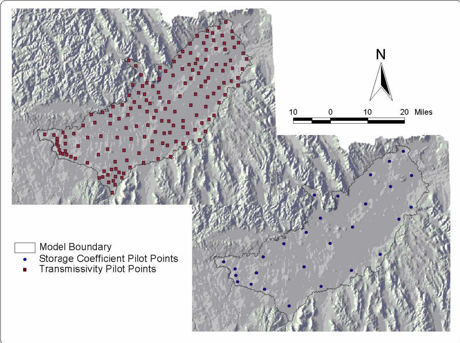
Figure 56. Location of pilot points used for calibration of transmissivity and aquifer storage.
