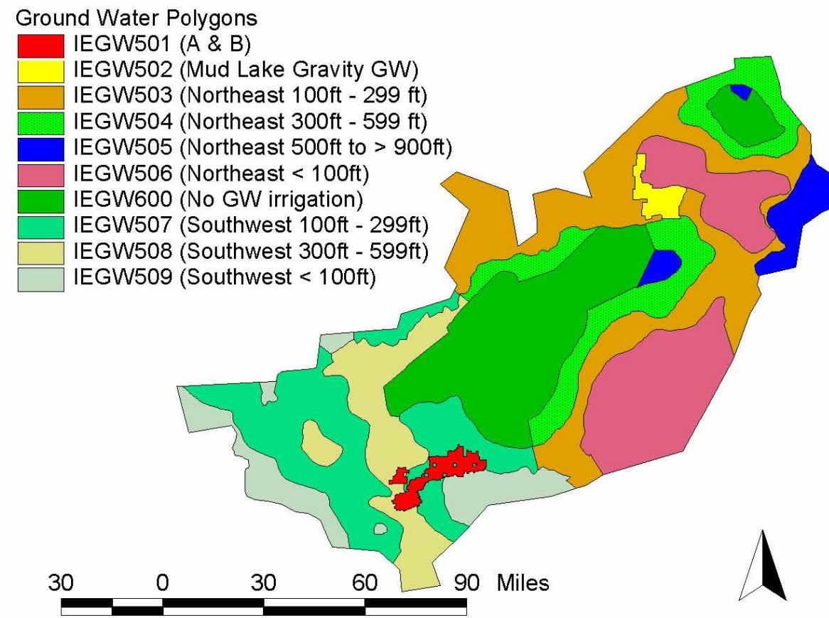
Figure 32. Ground-water polygons (based on depth to ground water).
