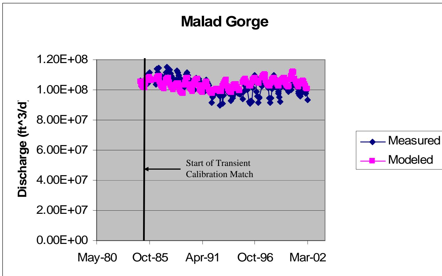
Figure 84. Modeled versus observed spring discharge—Malad ( $\text{ft}^3/\text{d}$ ).
