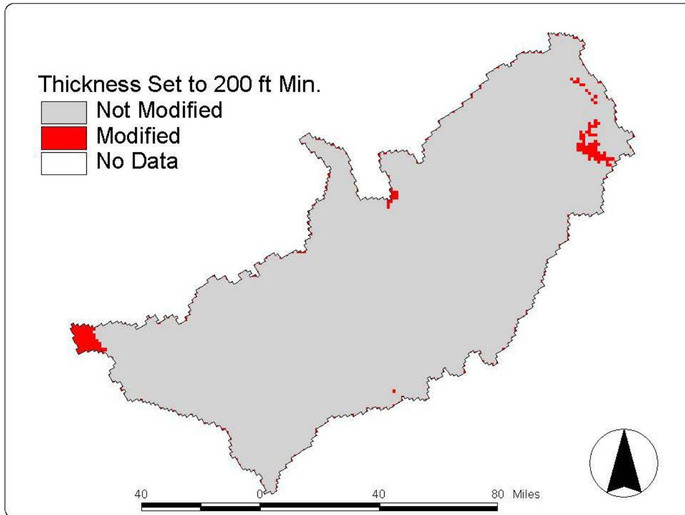
Figure 17. Areas where aquifer thickness was adjusted to 200 feet.
