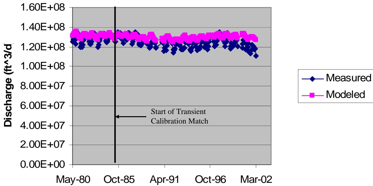
Figure 83. Modeled versus observed spring discharge—Thousand Springs (ft<sup>3</sup>/d).
