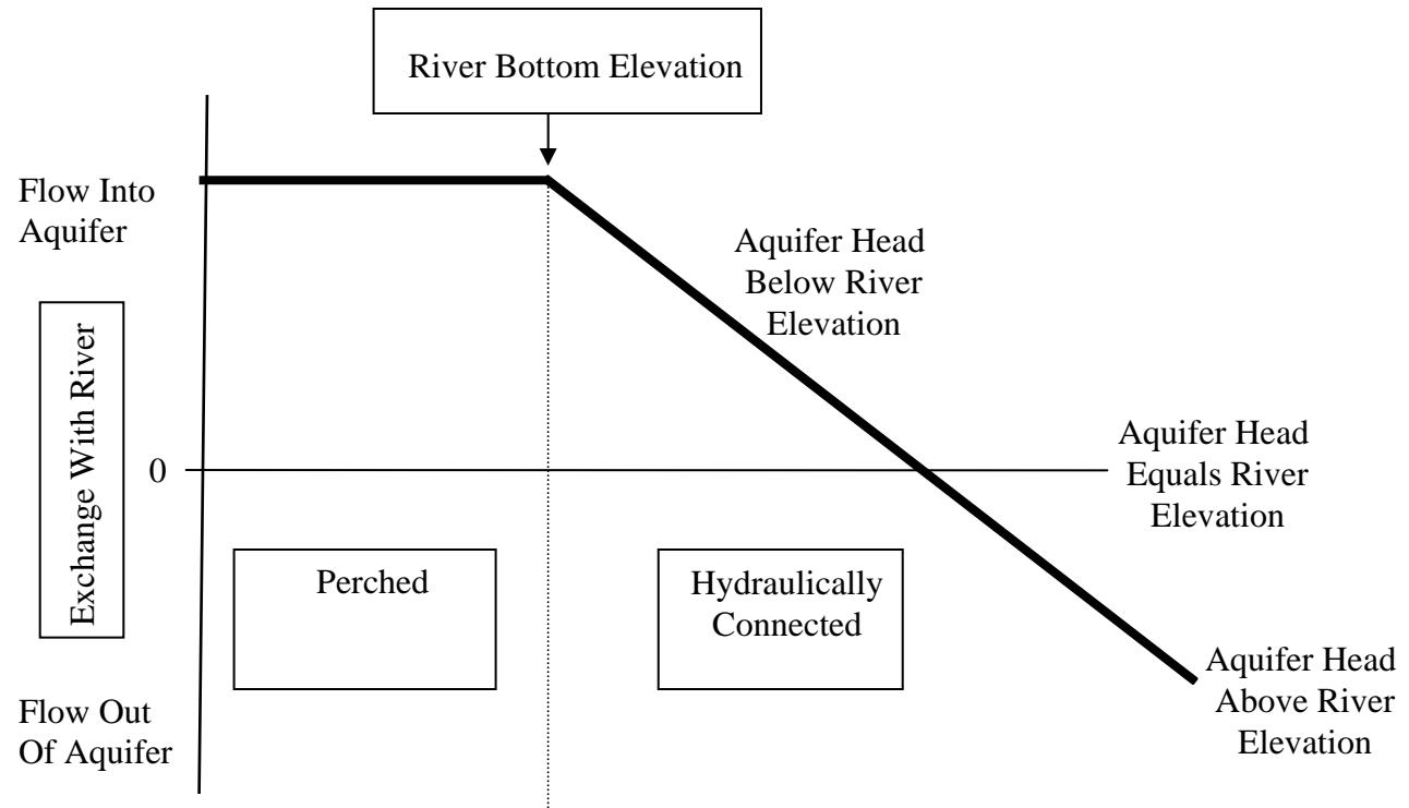
Figure 18. Conceptual illustration of river leakage computation
