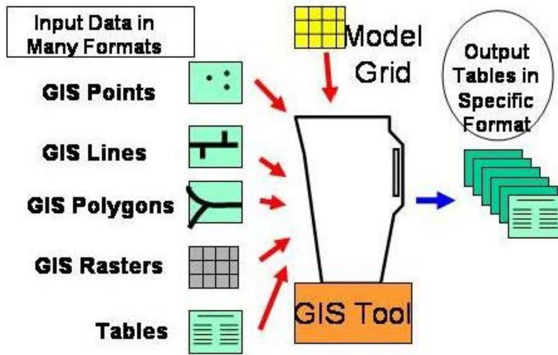
Figure B-1. Conceptual model of GIS component of the
