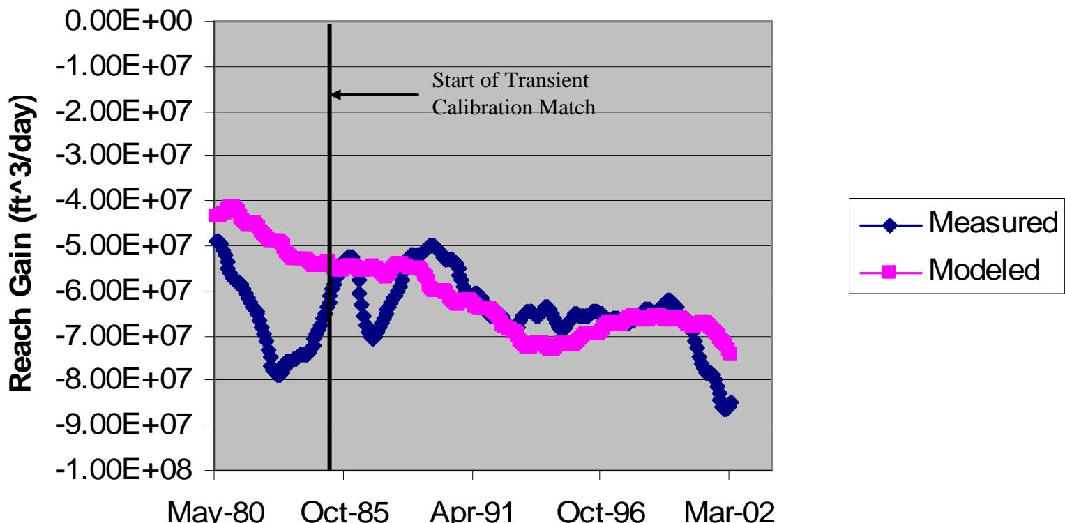
Figure 68. Modeled versus observed reach gain—Shelley to Near Blackfoot reach, filtered data.
