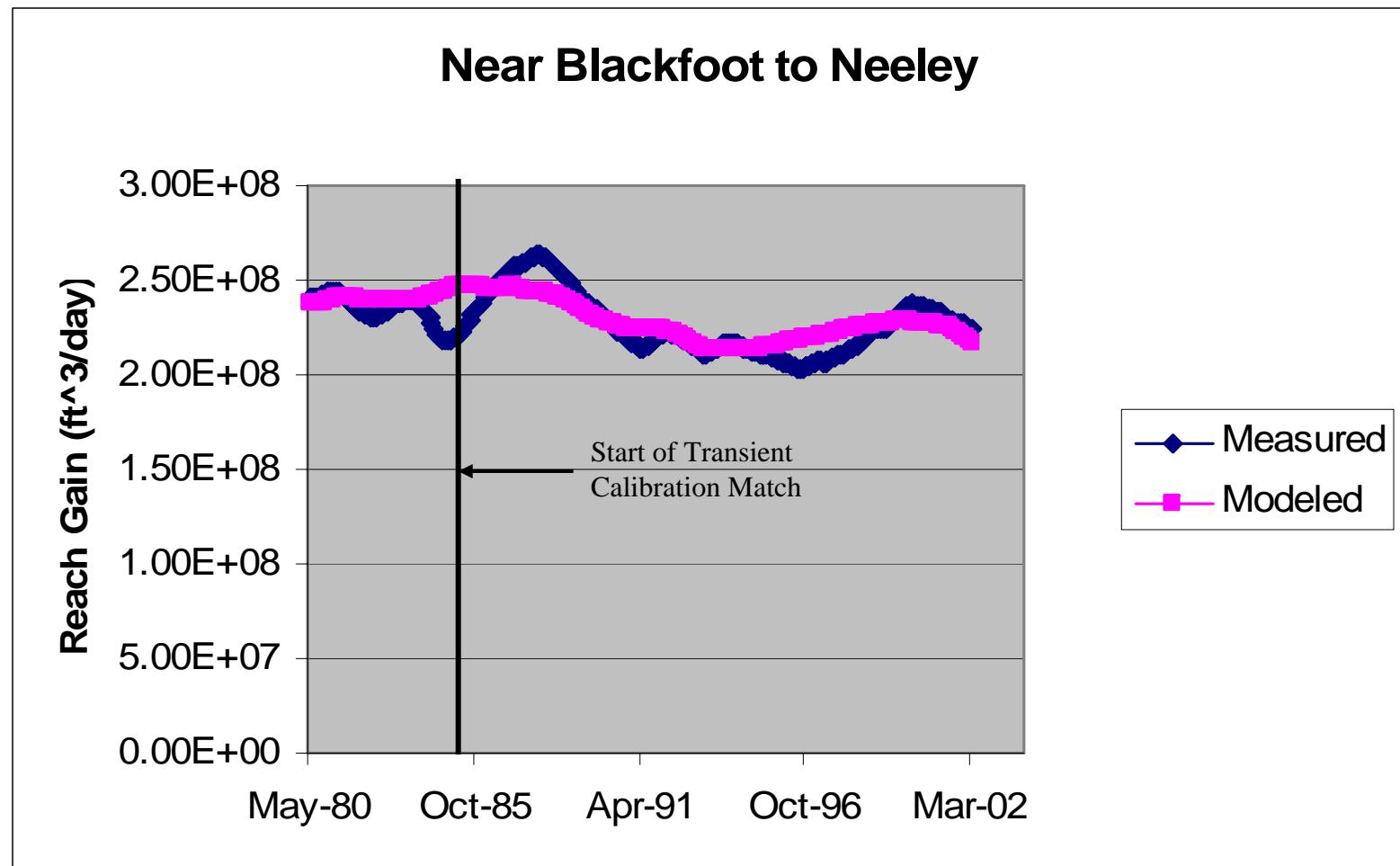
Figure 69. Modeled versus observed reach gain—Near Blackfoot to Neeley reach, filtered data.
