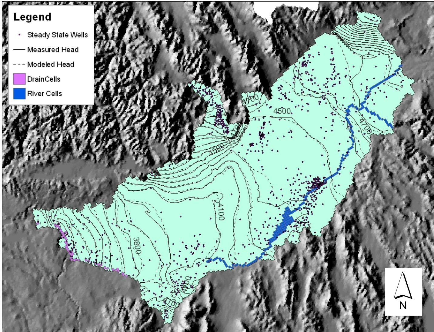
Figure 59. Steady state model-predicted versus observed aquifer potentiometric surface (100-ft. contours).
