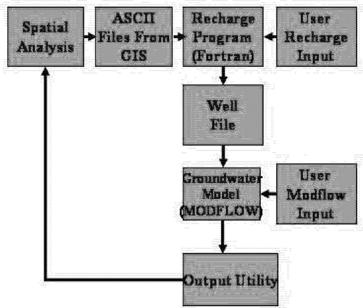
Figure B-7. Running the model without a parameter estimation routine. This schematic shows where the GIS and Fortran components of the recharge program fit in when running a model.
