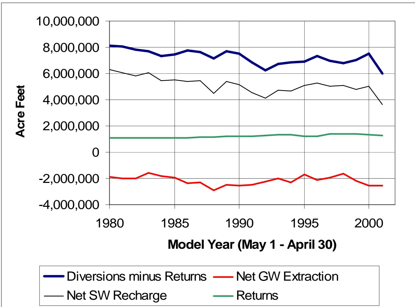
Figure 37. Diversion volume less return flow volume, return flow volume, net ground-water extraction and net recharge due to surface water irrigation.
