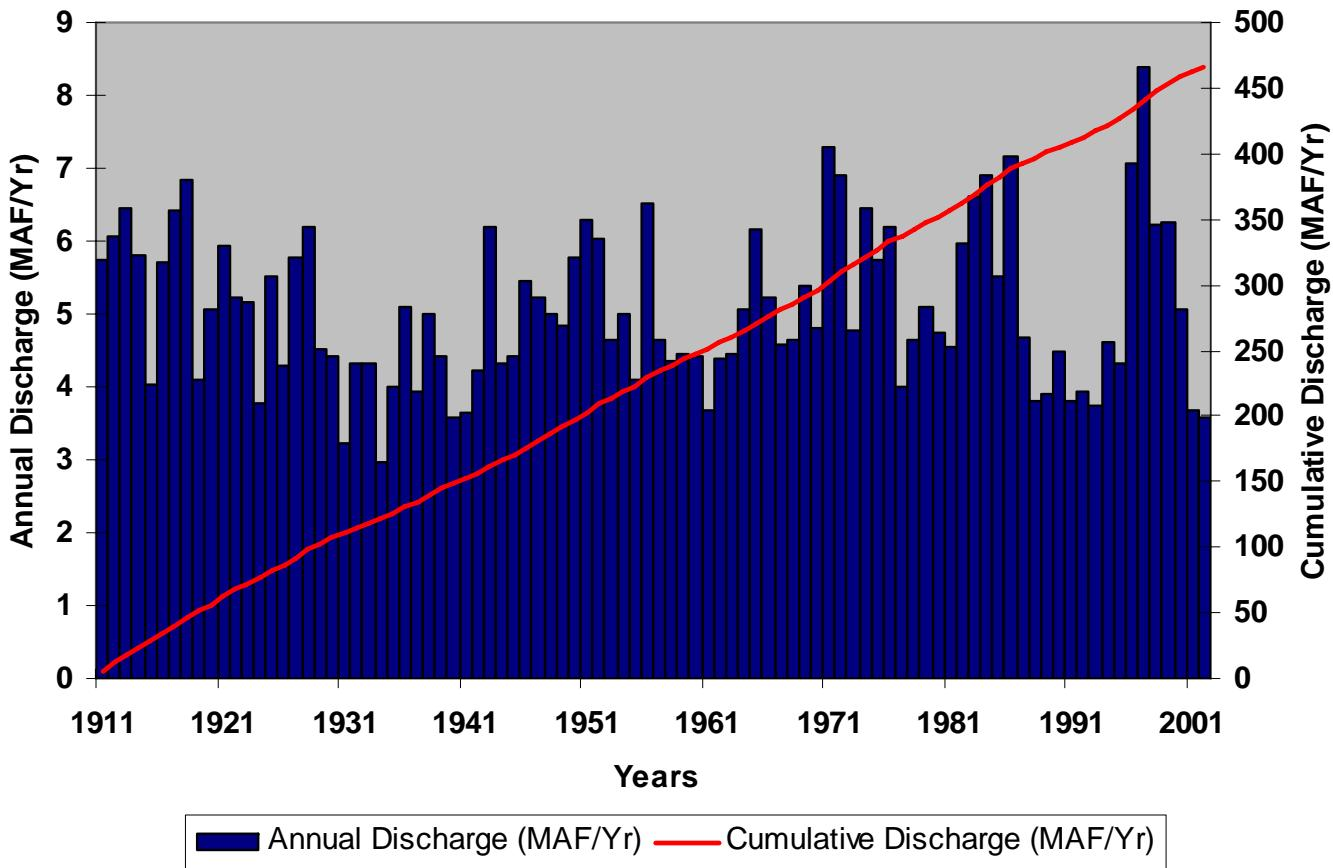
Figure 3. Annual and cumulative discharge of the Snake River near King Hill (U.S. Geological Survey data).
