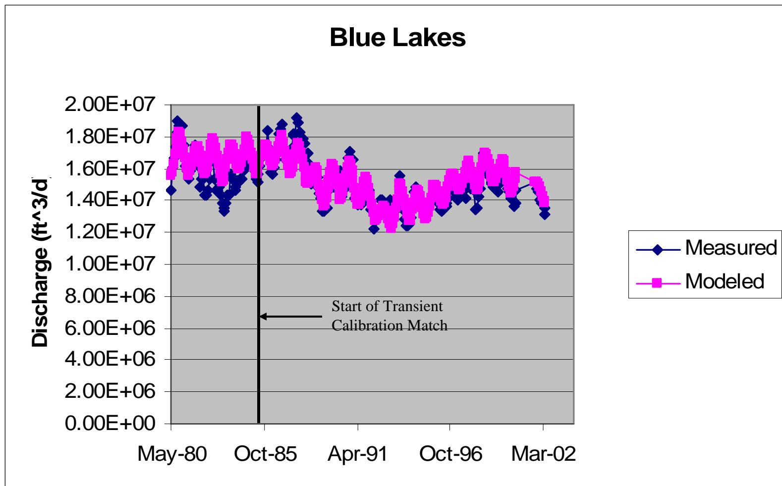
Figure 78. Modeled versus observed spring discharge—Blue Lakes ( $\text{ft}^3/\text{d}$ ).
