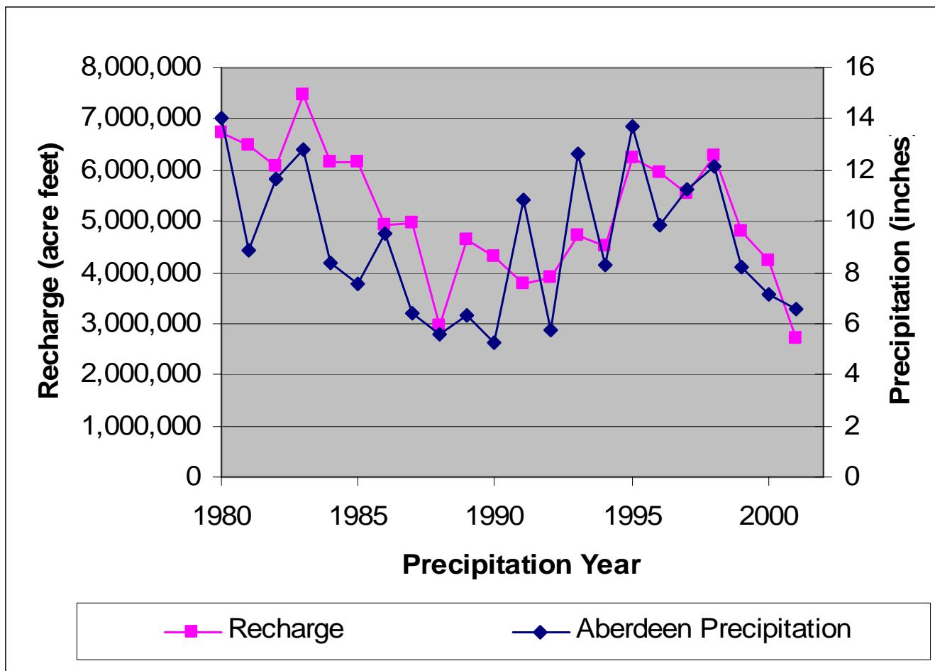
Figure 46. Recharge variation with time compared with precipitation at Aberdeen, Idaho for the transient ESPAM model.
