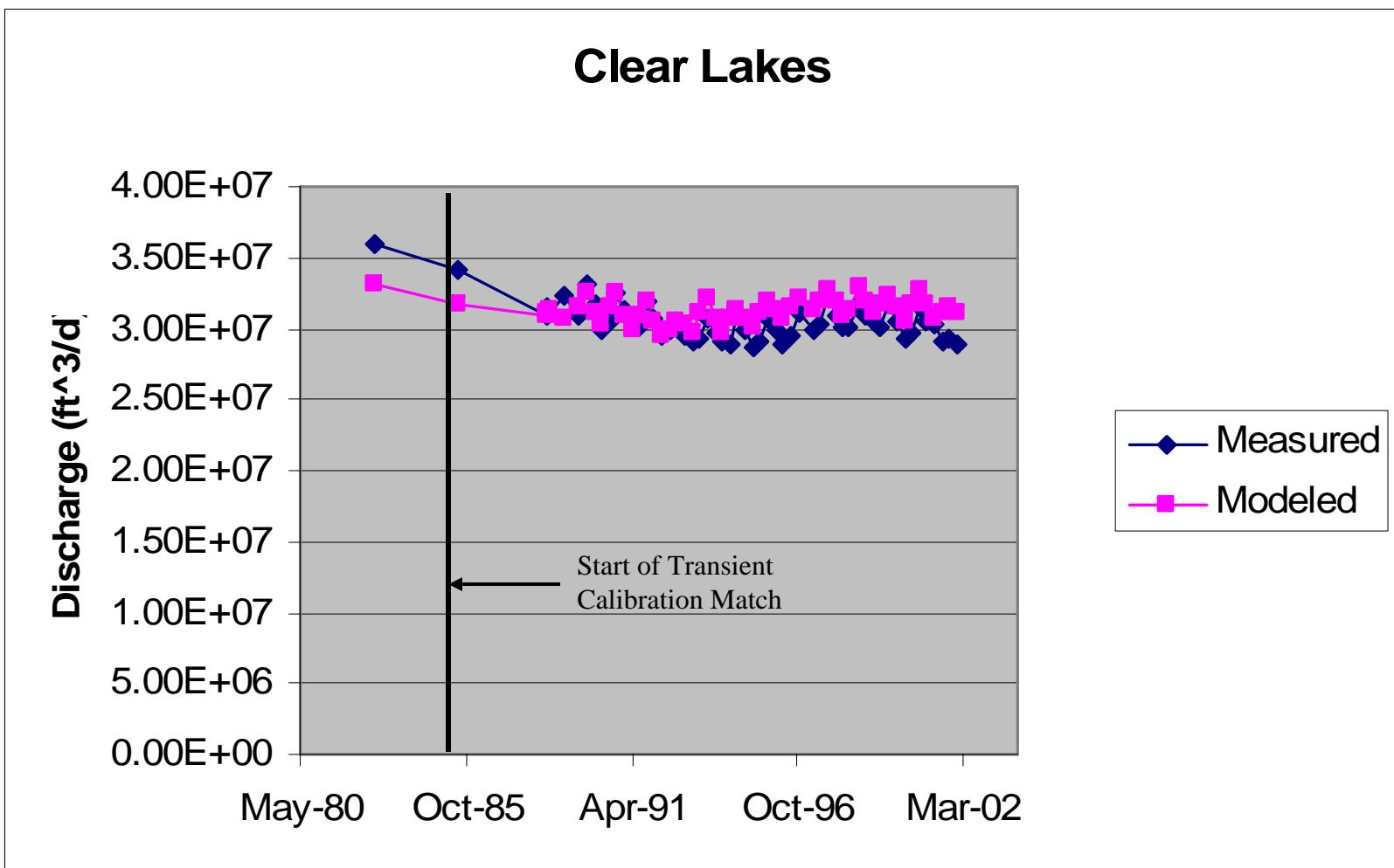
Figure 80. Modeled versus observed spring discharge—Clear Lakes (ft<sup>3/d</sup>).
