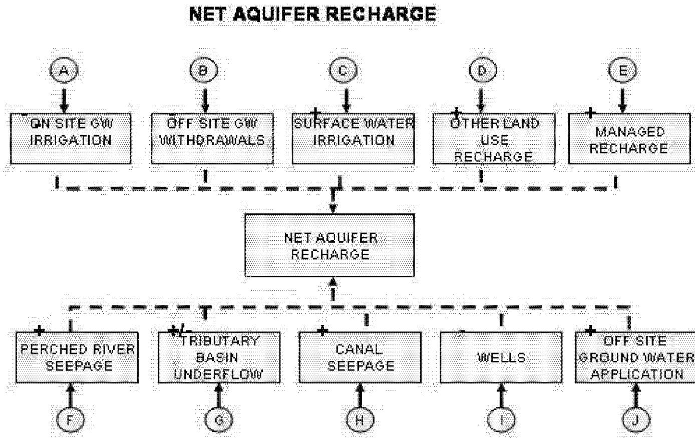
Figure B-2. Schematic of the components of recharge and discharge accounted for in the GIS/Fortran Recharge Tool.
