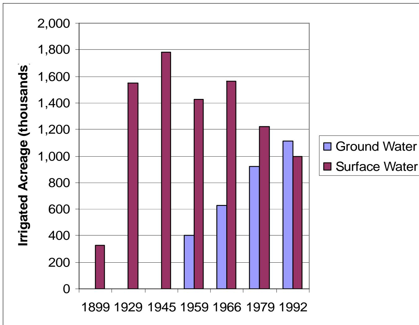
Figure 2. Changes in surface and ground water irrigated acres on the eastern Snake River Plain (after Garabedian, 1992).
