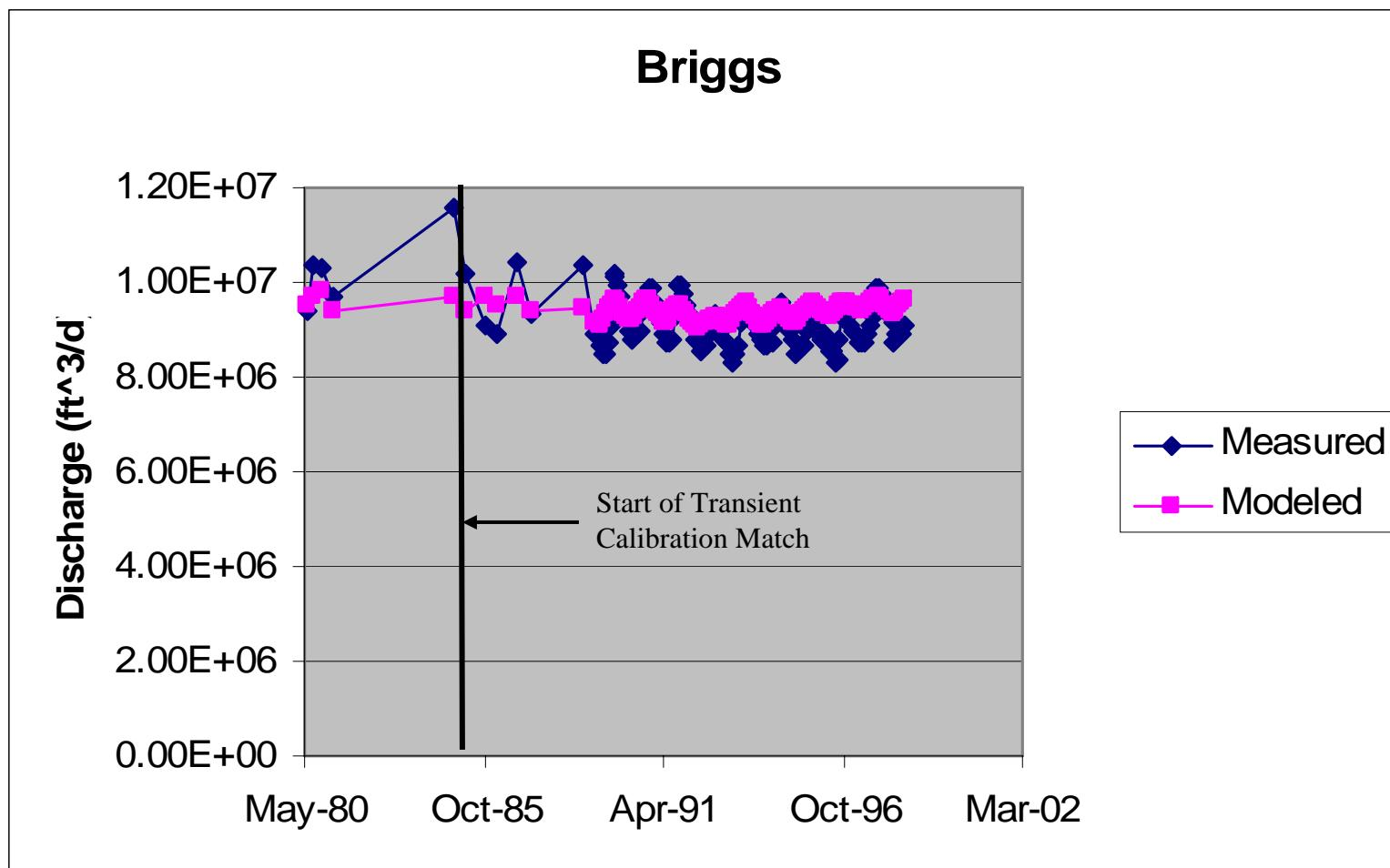
Figure 81. Modeled versus observed spring discharge—Briggs ( $\text{ft}^3/\text{d}$ ).
