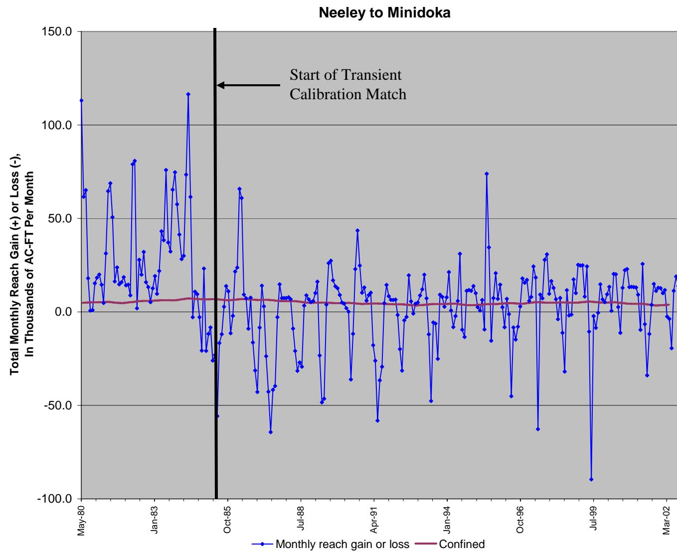
Figure 75. Modeled versus observed reach gain—Neeley to Minidoka reach, monthly unfiltered data.
