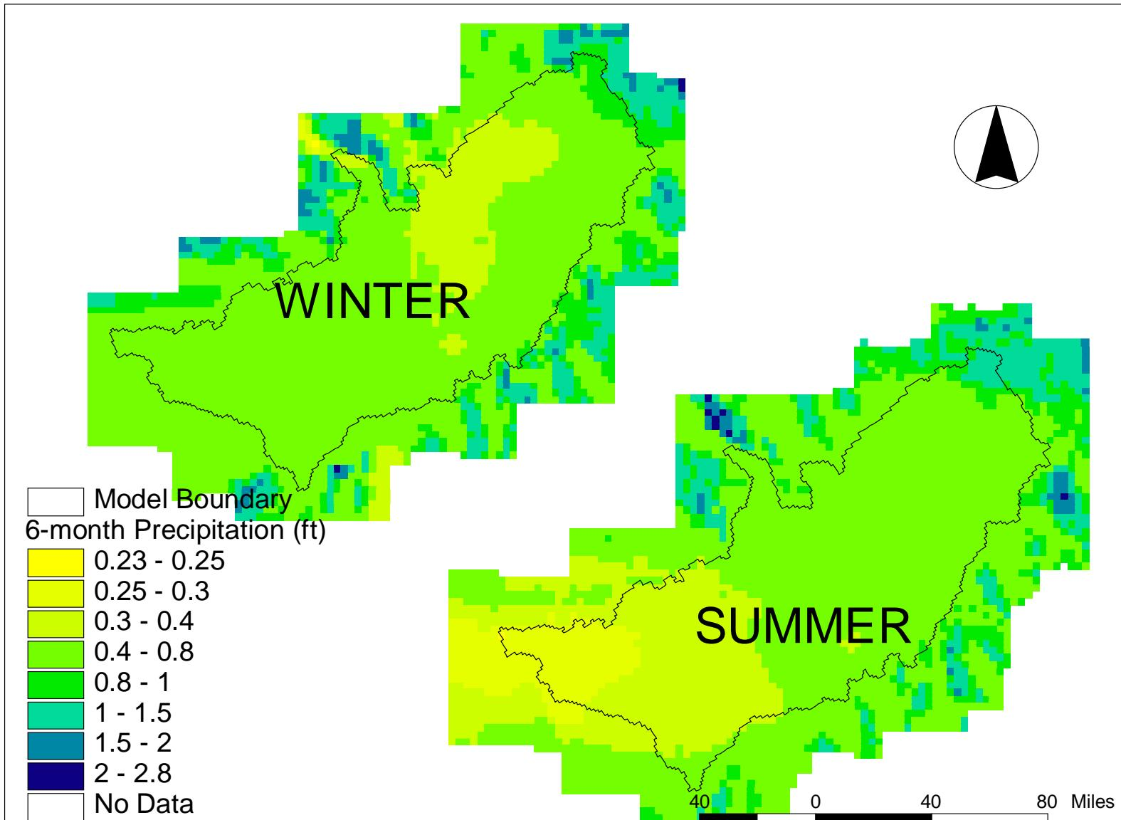
Figure 26. PRISM precipitation maps for the irrigation season and non-irrigation season, based on average precipitation for model period.
