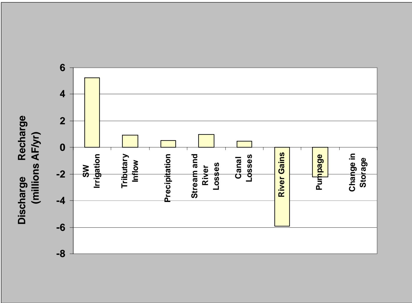
Figure 44. Bar graph of the components of recharge for steady state model.
