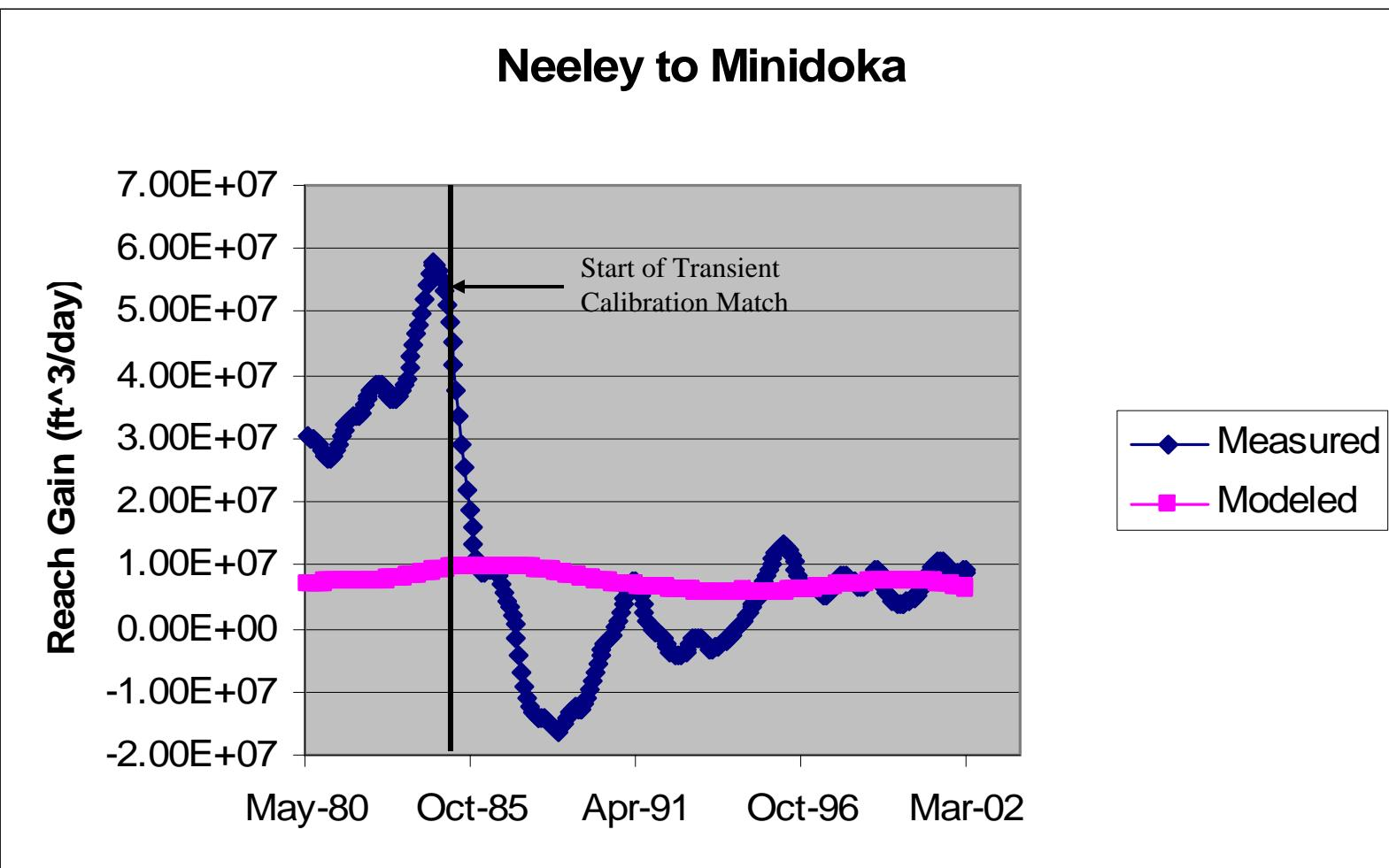
Figure 70. Modeled versus observed reach gain—Neeley to Minidoka reach, filtered data.
