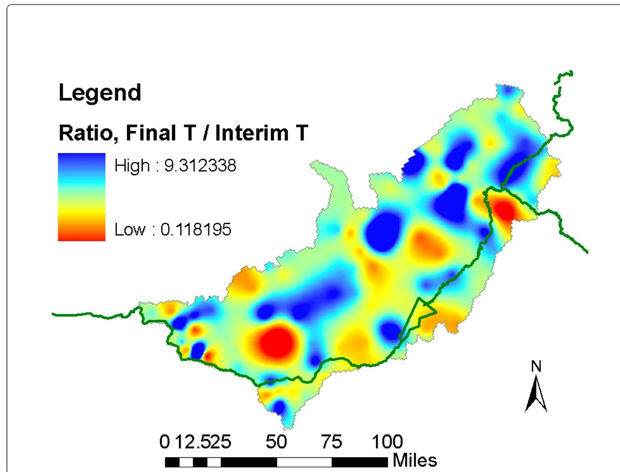
Figure 86. Ratio of final transmissivity to preliminary transmissivity.
