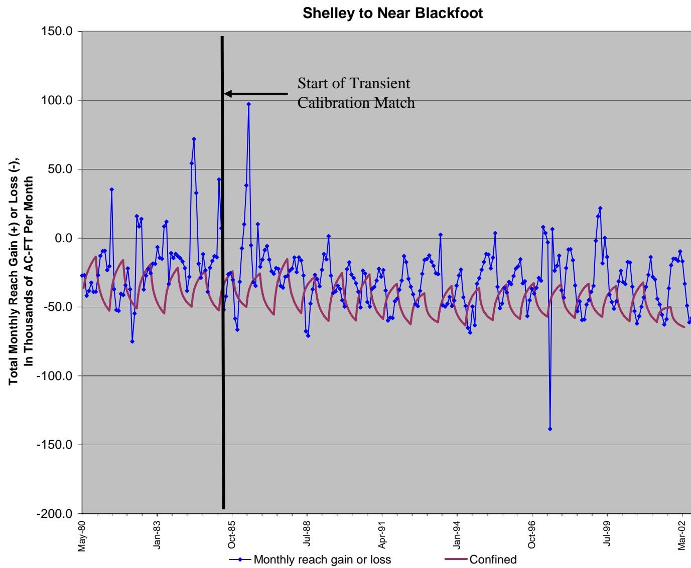
Figure 73. Modeled versus observed reach gain—Shelley to Near Blackfoot reach, monthly unfiltered data.
