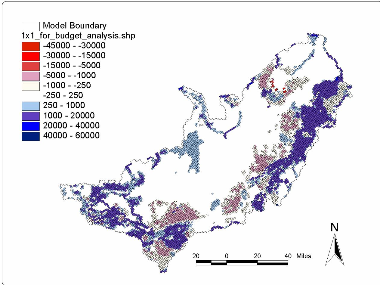
Figure 45. Areal distribution of recharge for steady state model (AF/yr).
