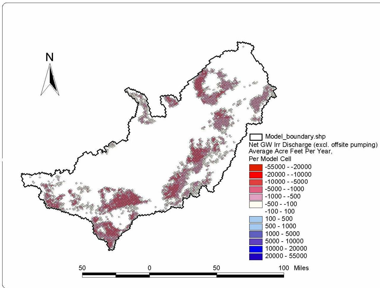
Figure 38. Areal distribution of net ground-water extraction averaged for the 22-year model calibration period.
