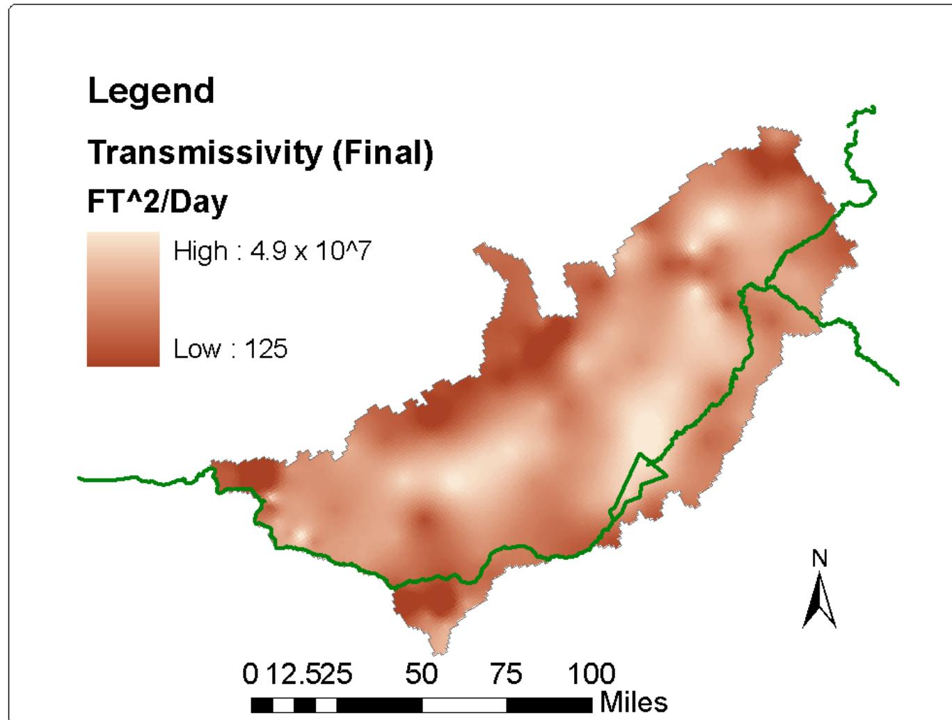
Figure 85. Transmissivity map from coupled steady state/transient calibration.
