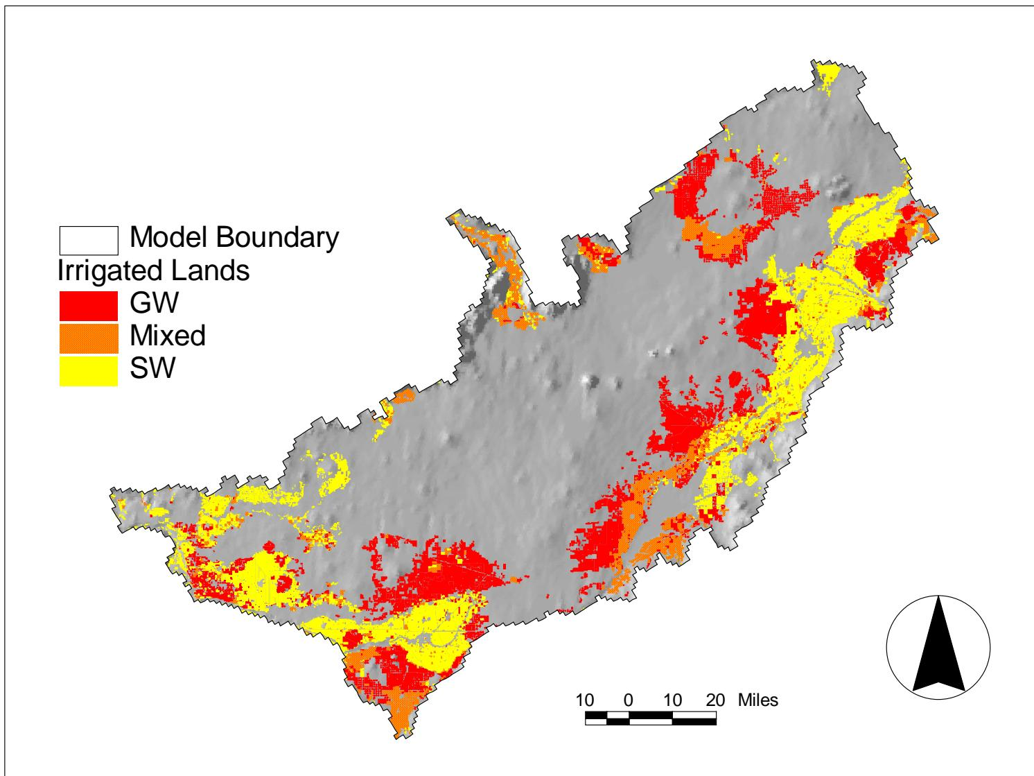
Figure 29. Irrigation water source determined from adjudication data.
