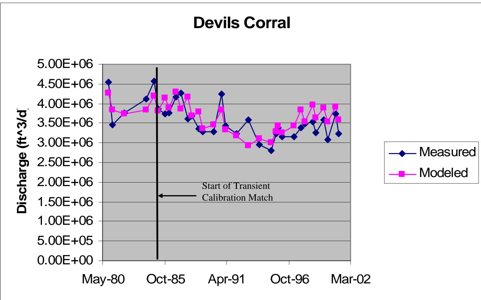
Figure 77. Modeled versus observed spring discharge—Devils Corral (ft<sup>3</sup>/d).
