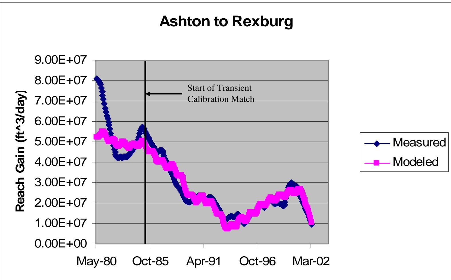
Figure 66. Modeled versus observed reach gain—Ashton to Rexburg reach, filtered data.
