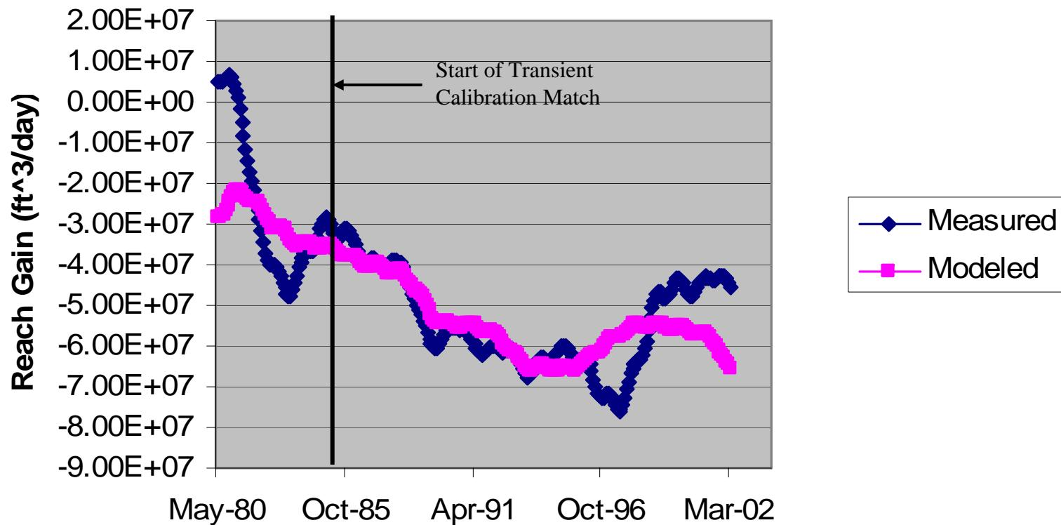
Figure 67. Modeled versus observed reach--Heise to Shelley reach, filtered data.
