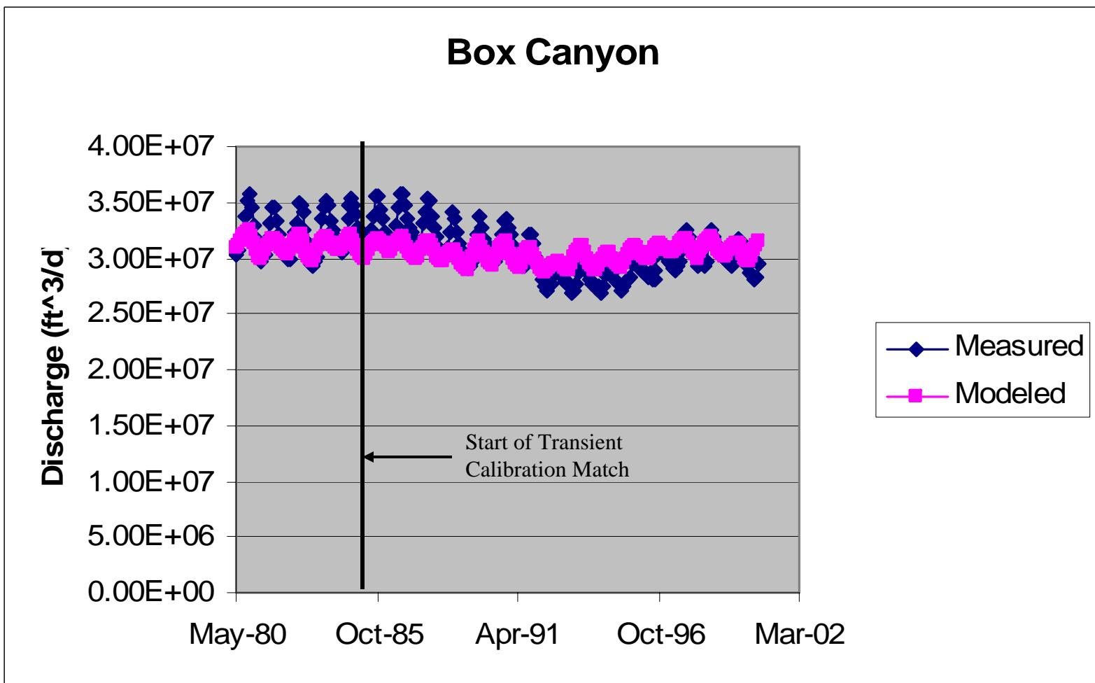
Figure 82. Modeled versus observed spring discharge—Box Canyon ( $\text{ft}^3/\text{d}$ ).
