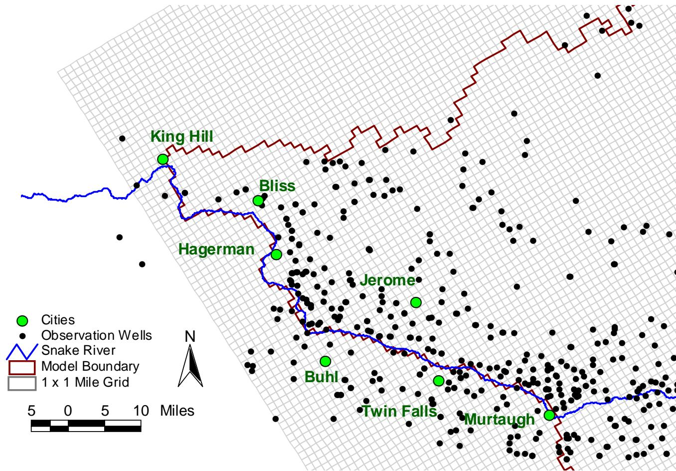
Figure 14. Close-up of model grid in the Thousand Springs area.
