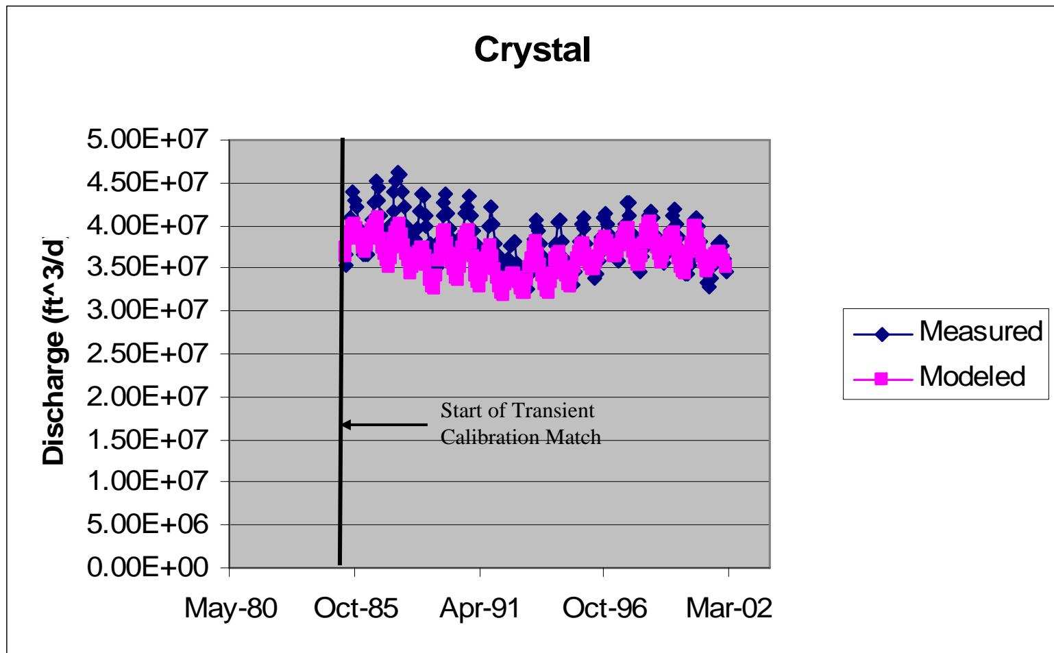
Figure 79. Modeled versus observed spring discharge—Crystal ( $\text{ft}^3/\text{d}$ ).
