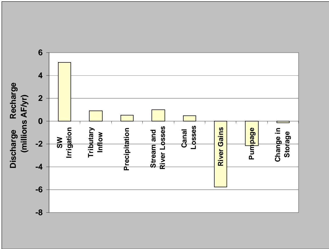
Figure 8. Snake River Plain Aquifer estimated annual recharge and discharge assuming the average irrigation development level of 1980 through 2001 (after IDWR, 1997).
