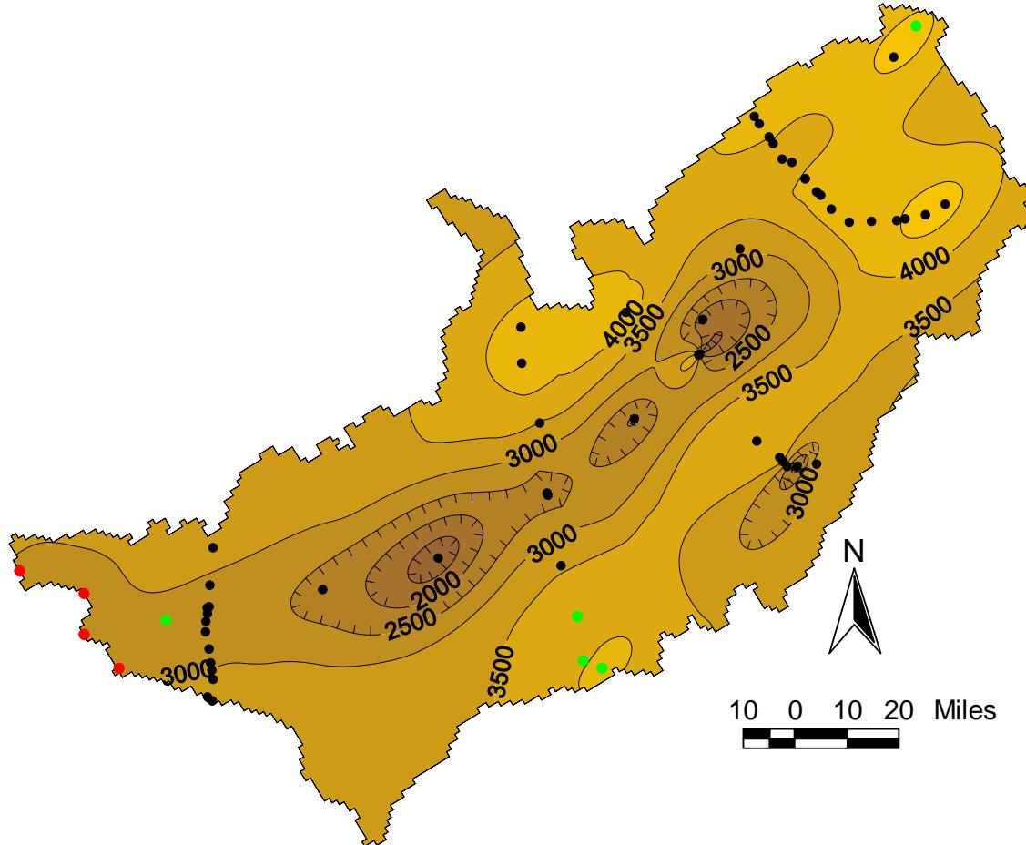
Figure 16. Aquifer bottom elevations with estimated elevation points. Based on modified Whitehead (1986) data. Black dots represent locations used by Whitehead, green dots represent modified Whitehead data points, red dots represent points added to anchor kriged surface.
