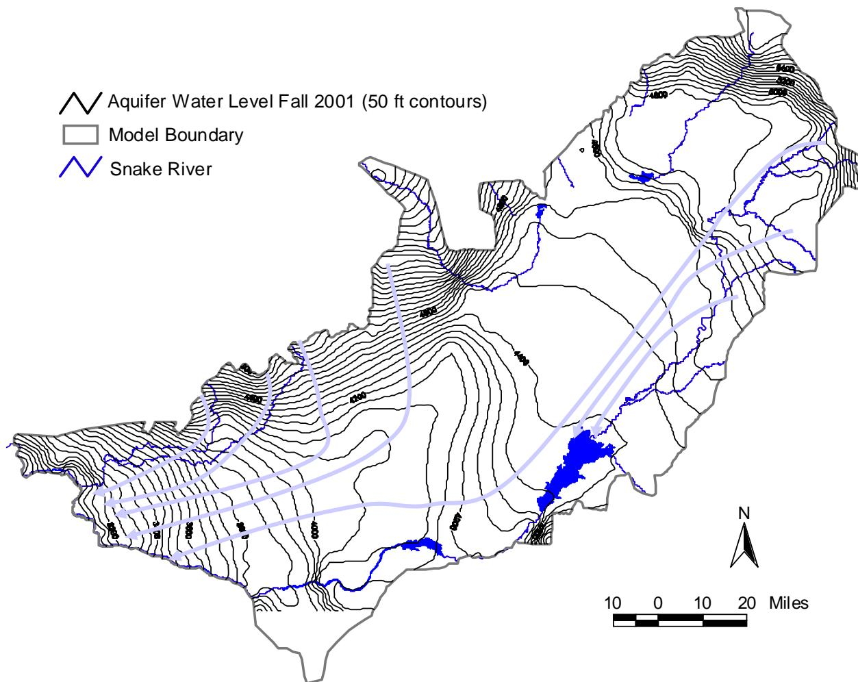
Figure 10. Contours of the Fall, 2001 potentiometric surface of the Snake River Plain Aquifer and estimated aquifer flow lines.
