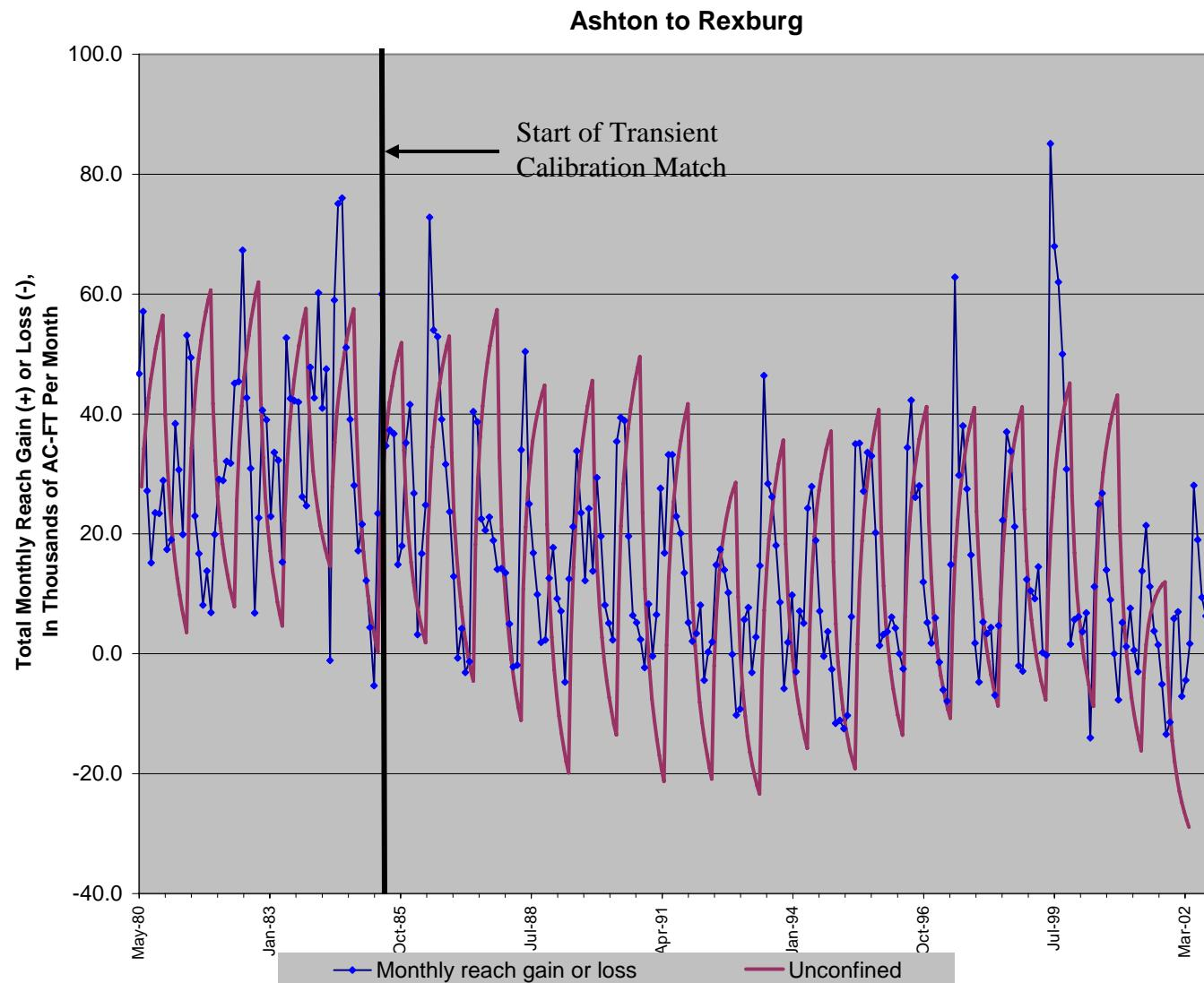
Figure 71. Modeled versus observed reach gain—Ashton to Rexburg reach, monthly unfiltered data.
