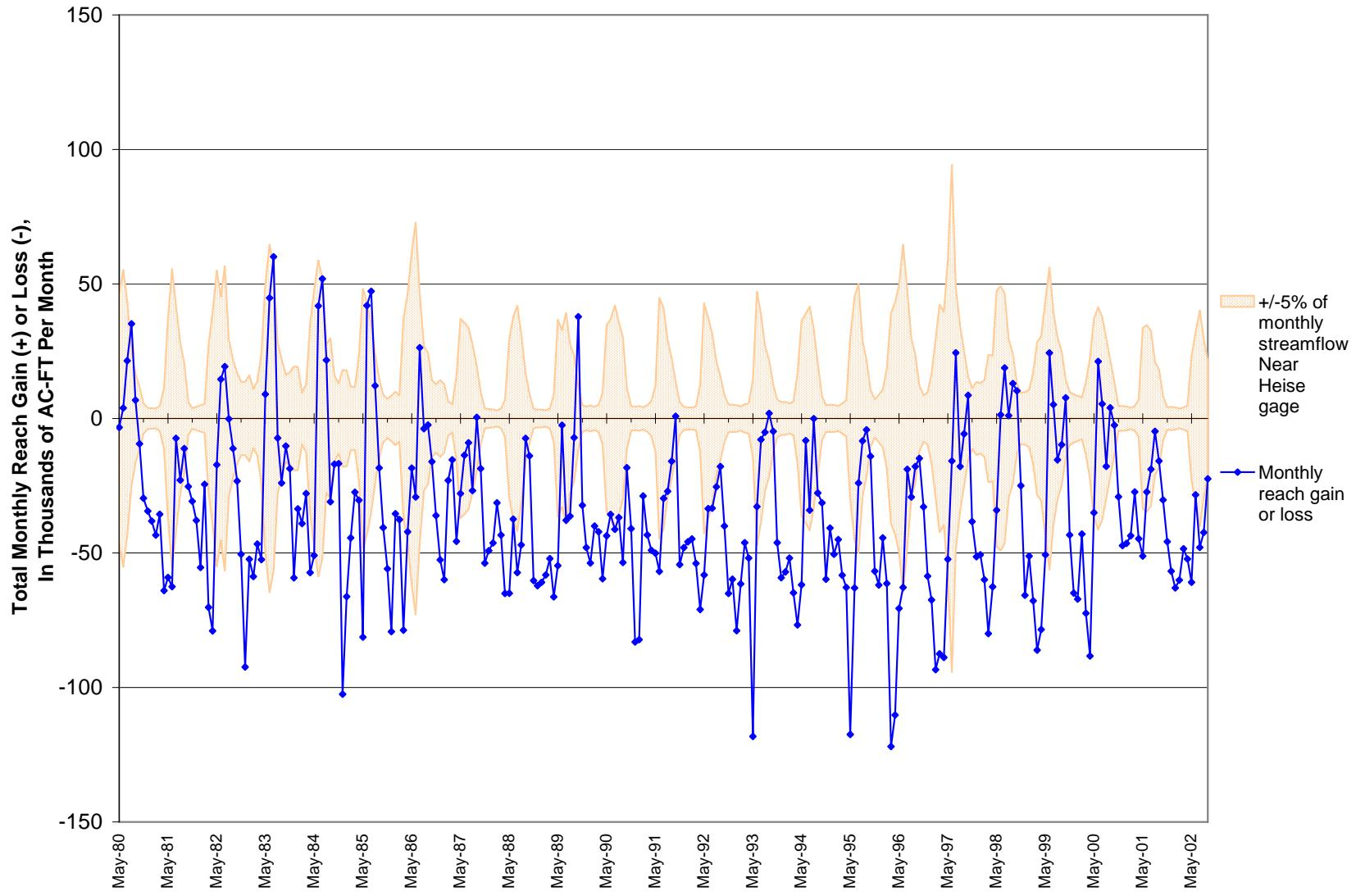
Figure 50. Monthly Snake River gains and losses: Heise to Shelley reach.
