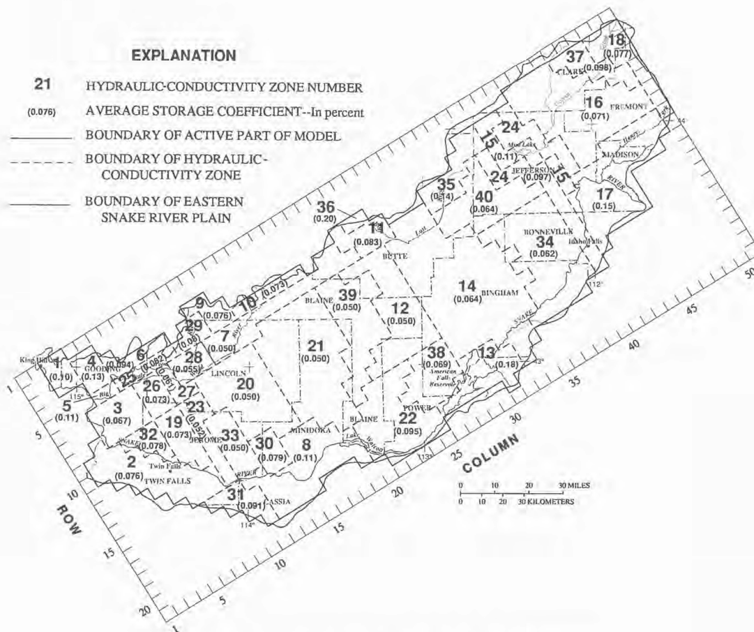
FIGURE 24.—Hydraulic-conductivity zones and average storage coefficients, model layer 1.
