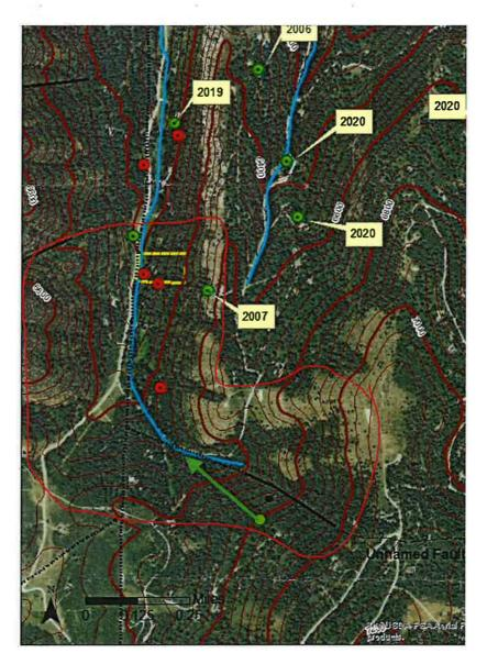
Proposed boundary for area having a common ground water supply is delineated with the thin red line.
