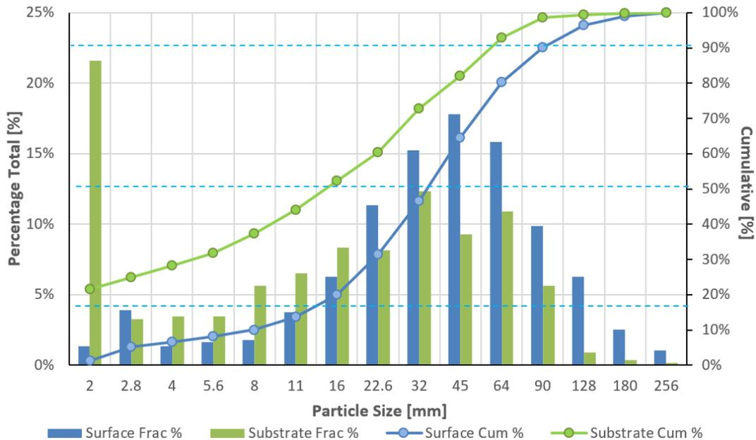
Figure 25. Surface and substrate particle size distribution and cumulative percent finer used in the Ellsworth study reach computations. Dashed lines represent  $D_{16}$ ,  $D_{50}$ , and  $D_{90}$ . Source data: UI-CER 2020.
