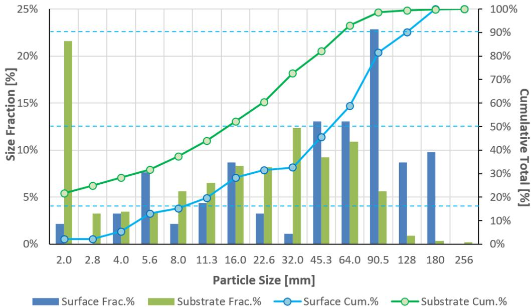
Figure 29. Surface and substrate particle size distribution and cumulative percent finer used in the L-46 study reach computations. Dashed lines represent  $D_{16}$ ,  $D_{50}$ , and  $D_{90}$ . Source data: UI-CER 2020.
