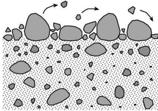
Figure 8. Schematic riverbed cross-section of an armored layer atop a finer substrate (Bunte & Abt 2001).
