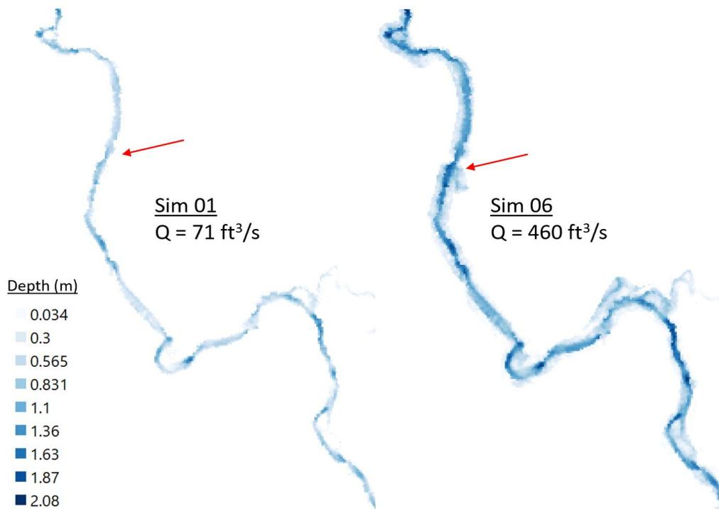
Figure 16. Simulated depths of the Lemhi River up and downstream of the LR-MC gauge (red arrow) for Sim01 and Sim06. Note, the depth color scale represents Sim06, but Sim01 uses a similar scale.
