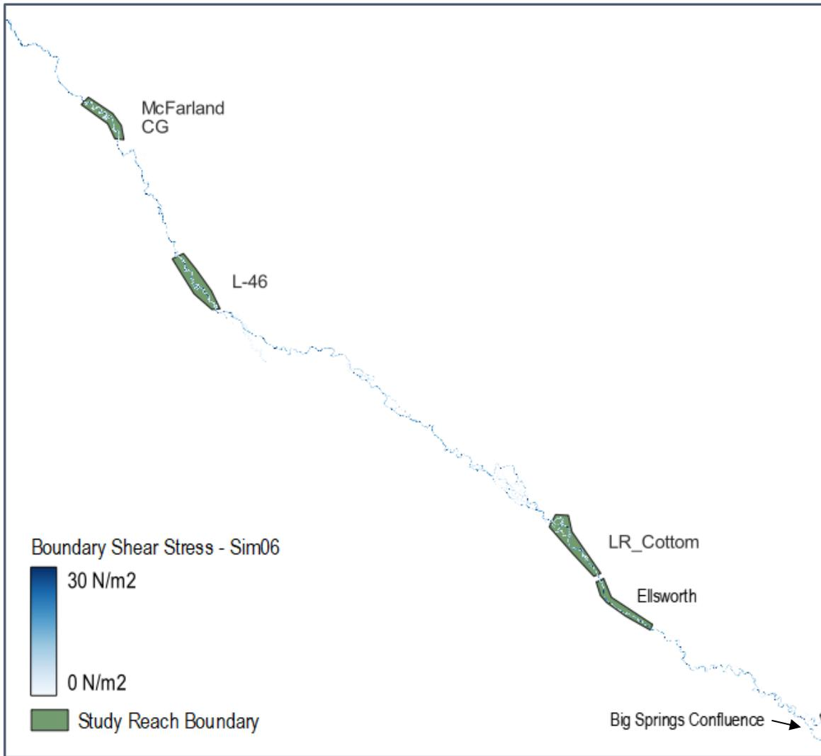
Figure 13. Lemhi River study reaches and boundary shear stress from UI-CER Sim06.
