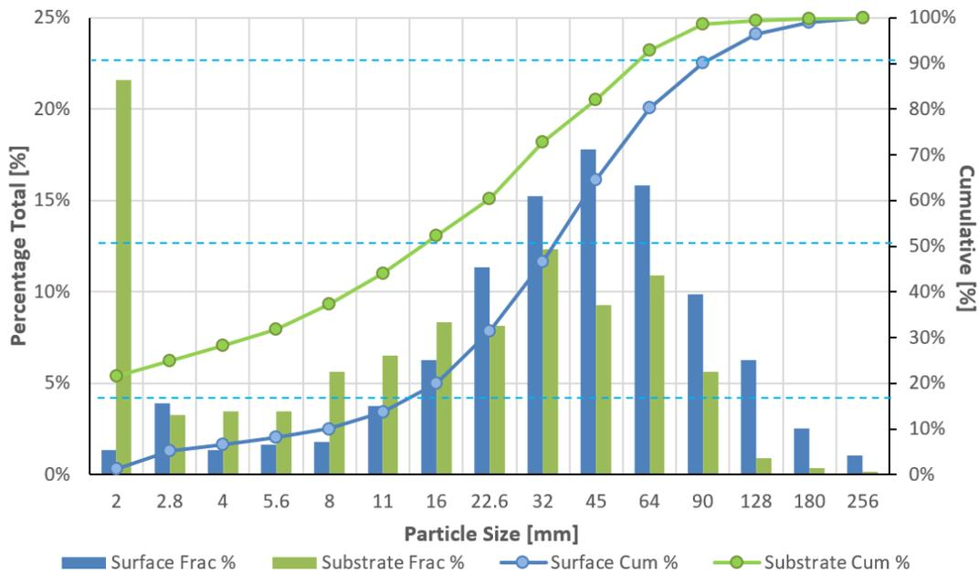
Figure 27. Surface and substrate particle size distribution and cumulative percent finer used in the Cottom Lane study reach computations. Dashed lines represent  $D_{16}$ ,  $D_{50}$ , and  $D_{90}$ . Source data: UI-CER 2020.
