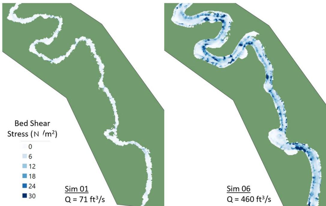
Figure 17. Boundary shear stress in the LR-MC reach from the UI-CER 2D hydrodynamic model for Sim01 and Sim06.
