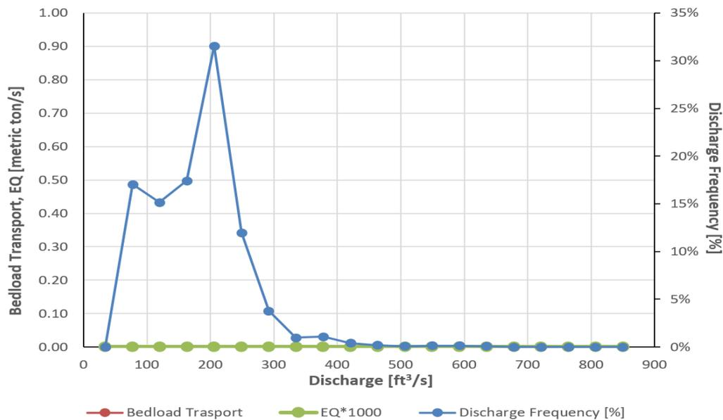
Figure 19. Effective discharge (EQ) calculated at LR-MC study reach.
