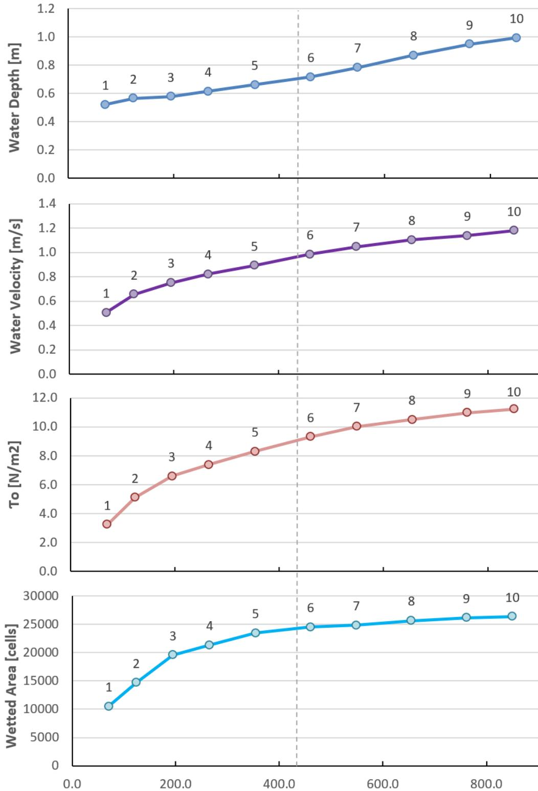
Figure 15. LR-MC reach average water depth, velocity, boundary shear stress ( $T_o$ ) as well as wetted area from the 2D hydrodynamic model simulations (1-10). Target discharge is denoted by the vertical dashed grey line.
