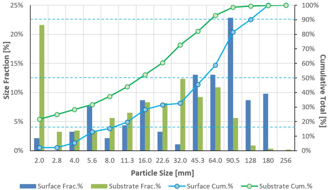
Figure 14. Particle size distribution and cumulative percent finer for the surface and substrate materials in the LR-MC. Dashed lines represent  $D_{16}$ ,  $D_{50}$ , and  $D_{90}$ . Source data: UI-CER 2020.
