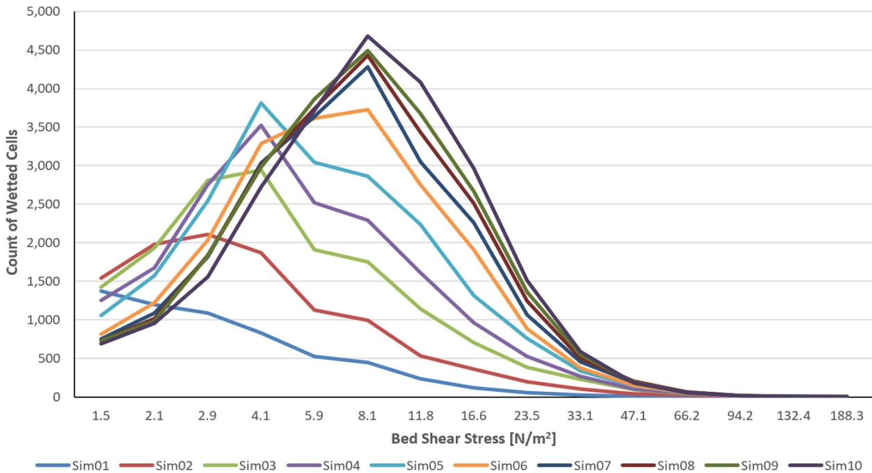
Figure 18. Count of wetted cells (proxy for area) by boundary shear stress for the LR-MC reach. Note the boundary (bed) shear stress values correspond to the incipient motion shear stress for particle sizes without shielding effect.
