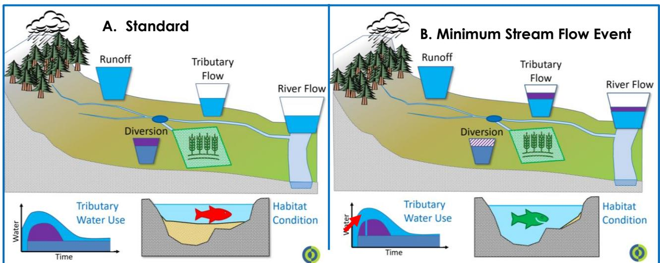
Figure 1. Schematics illustrating diversion practices during Spring runoff for (A) standard irrigation and (B) minimum stream flow event. Red arrow in 1B is points to the gap in high water diversion (purple) when the Lemhi River minimum stream flow event is in operation during the irrigation season.
