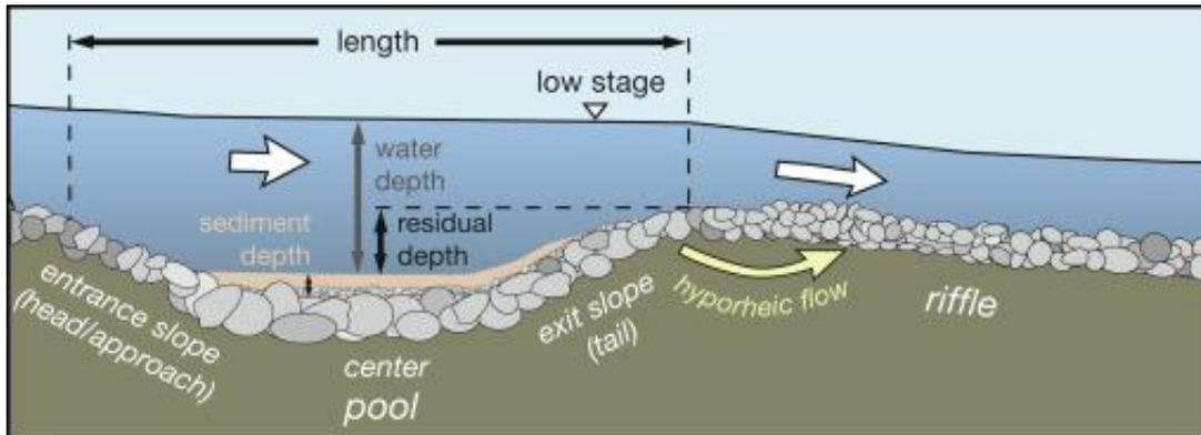
Figure 6. Diagram of a pool-riffle sequence illustrating deposition of fines in the pool and clean gravels in the riffles (source: Thompson 2018).
