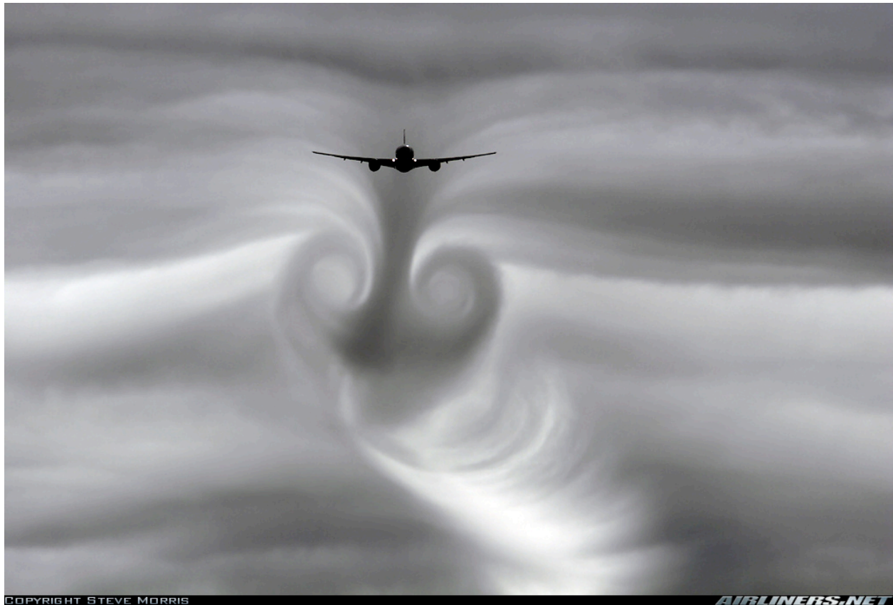
1 2 FIG. 3. Downwash and vortex pair below a B-777-200 aircraft (estimated mass 1.45 \times 10^5 kg) 3 flying immediately above a 150 m thick cloud while approaching London Gatwick airport at 4 7AM local daylight time on 10 July 2006. Surface temperature was 16^\circ\text{C} . Aircraft was 5 descending through an altitude of 0.61 km at a speed of about 108\text{ m s}^{-1} . Photograph courtesy of 6 Steve Morris photographer, who was positioned about 9 km in front of the approaching aircraft 7 at the surface, using a 840mm telephoto lens. Cloud in this viewing area was reported to 8 completely dissipate 20 minutes after the photograph was taken. It is suggested here that these 9 aircraft-scale vortices can under many conditions laterally propagate via the release of cloud-top 10 entrainment instability, dissipating by evaporation much larger cleared tracks shown in Figs. 1-2.
