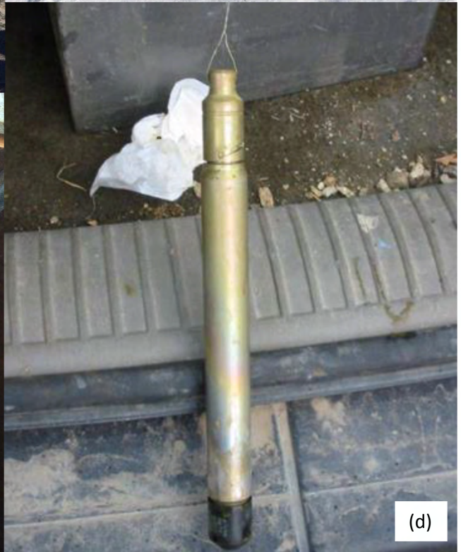
ATTACHMENT B: Photographs of (a) well drilling, (b) the completed well, (c) installed groundwater telemetry equipment, and (d) a water level pressure transducer.
