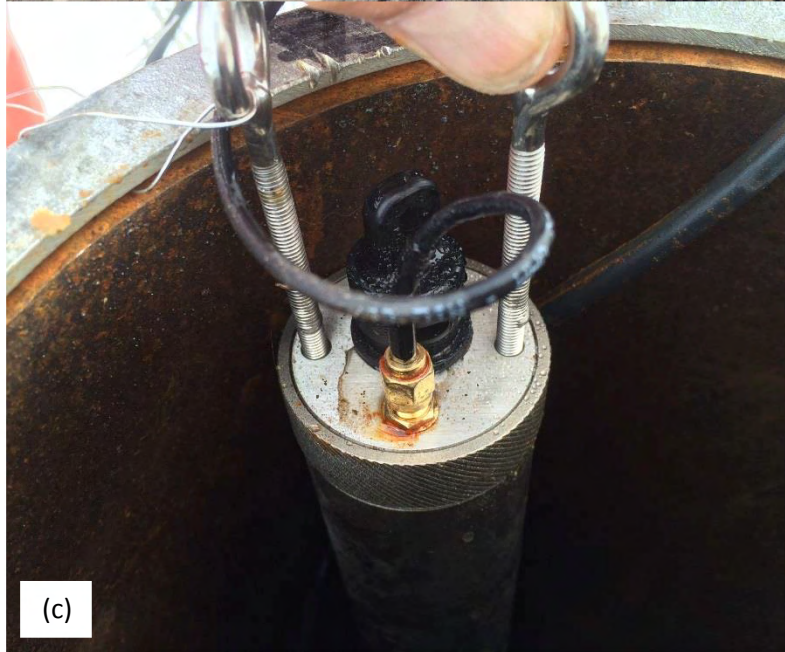
ATTACHMENT B: Photographs of (a) well drilling, (b) the completed well, (c) installed groundwater telemetry equipment, and (d) a water level pressure transducer.
