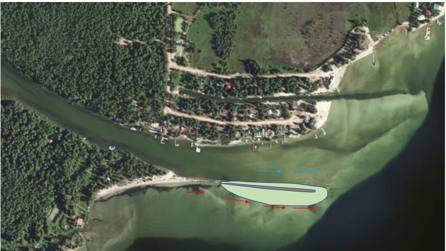
Replace Existing Porous Breakwater with Sediment Retention Feature
