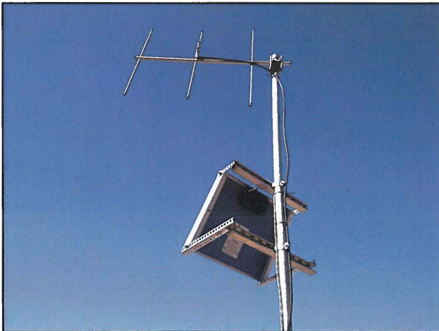
SV Ranch 1 Yagi 3 element 7.5dB Directional Antenna
