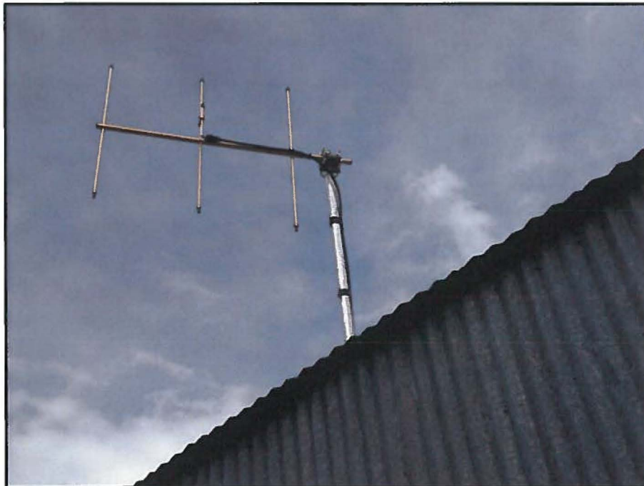
Robert Meyers Yagi 3 element 7.5 dB antenna
