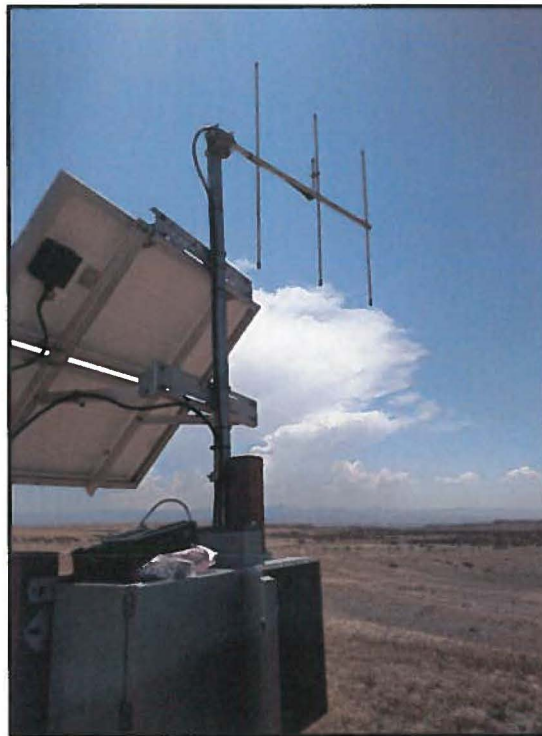
Owyhee Farms Snake River Yagi 3 element 7.5 dB antenna
