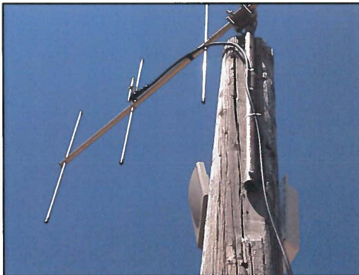
Owyhee Farms Black Sands Yagi 3 element 7.5 dB antenna
