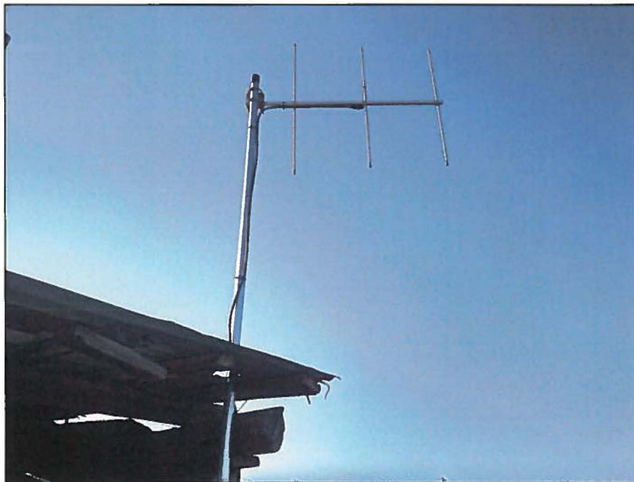
Quey Johns Yagi 3 element 7.5 dB antenna
