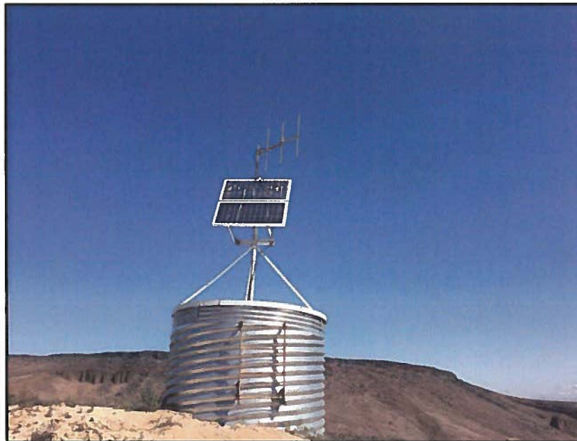
Dale Van Es CMP, solar panel, and Yagi 3 element 7.5dB antenna
