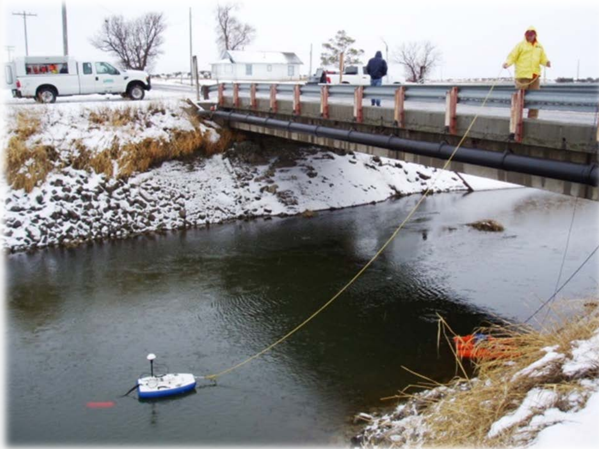
Measuring recharge flow in Milner- Gooding Canal January 16, 2015
