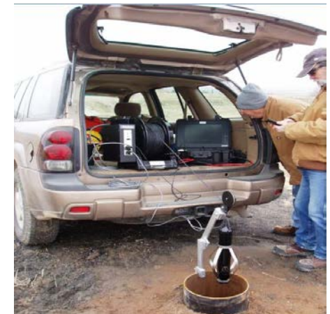
LSRARD and Idaho Power assisting IDWR staff with borehole camera Milner Reservoir test well.
