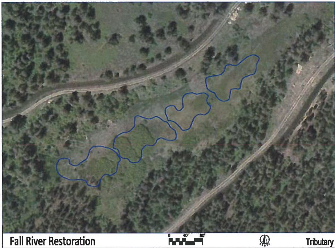
Figure 40. Overlay of plan view layout of the proposed linked beaver dam ponds.
