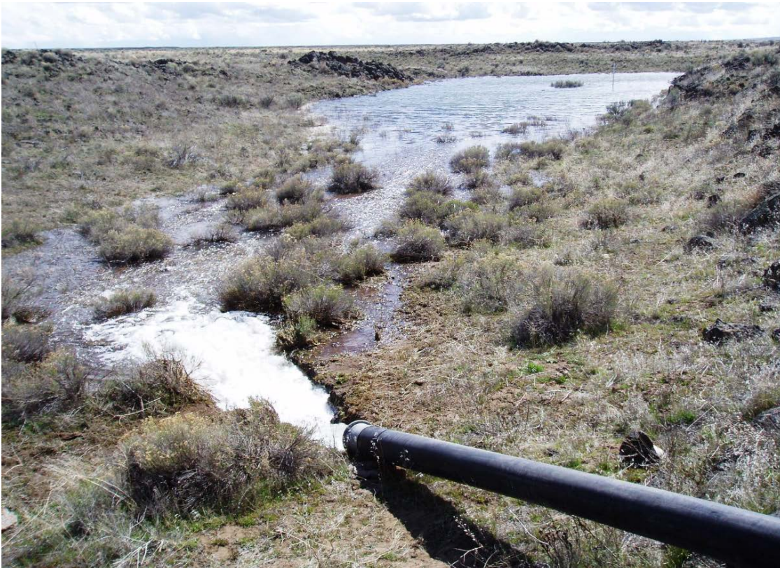
Discharge into Richfield site test basin at 4.8 cfs.
