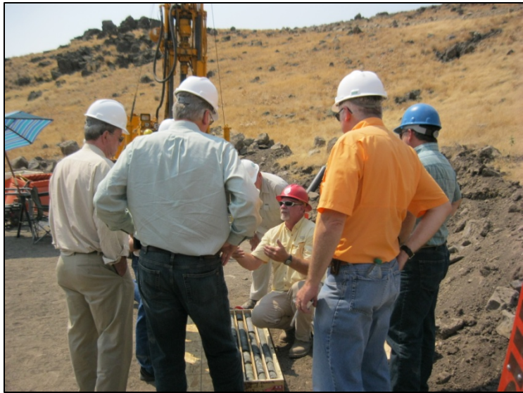
Photo: IWRB members examining core drilling investigation work at the proposed Galloway dam site to determine the site's suitability for development of a large dam and reservoir project.
