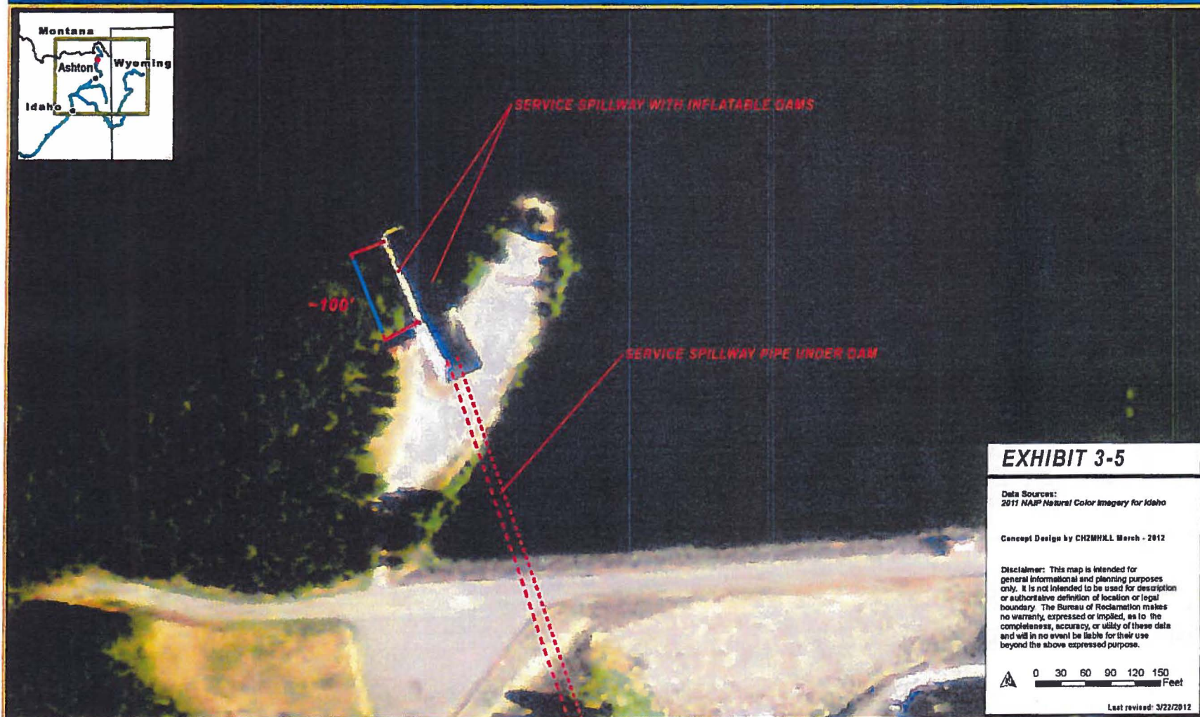
EXHIBIT 3-5 Island Park Dam Raise Alternative: Service Spillway
