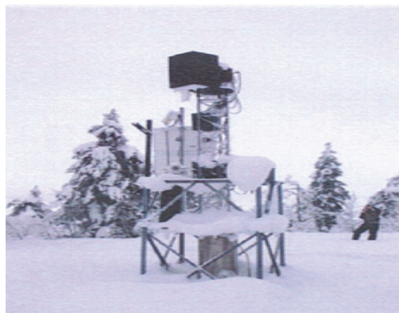
Remote-operated cloud seeding generator located at Antelope Flat.
