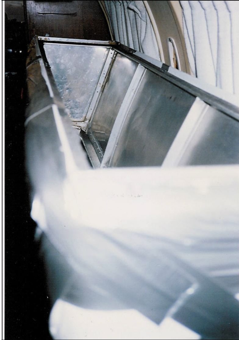
Figure 3.10 Dry Ice Dispenser Mounted in a Seeding Aircraft
