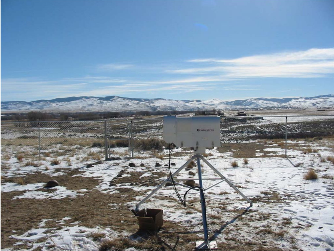
Figure 8.2 Example of a Portable Microwave Radiometer
