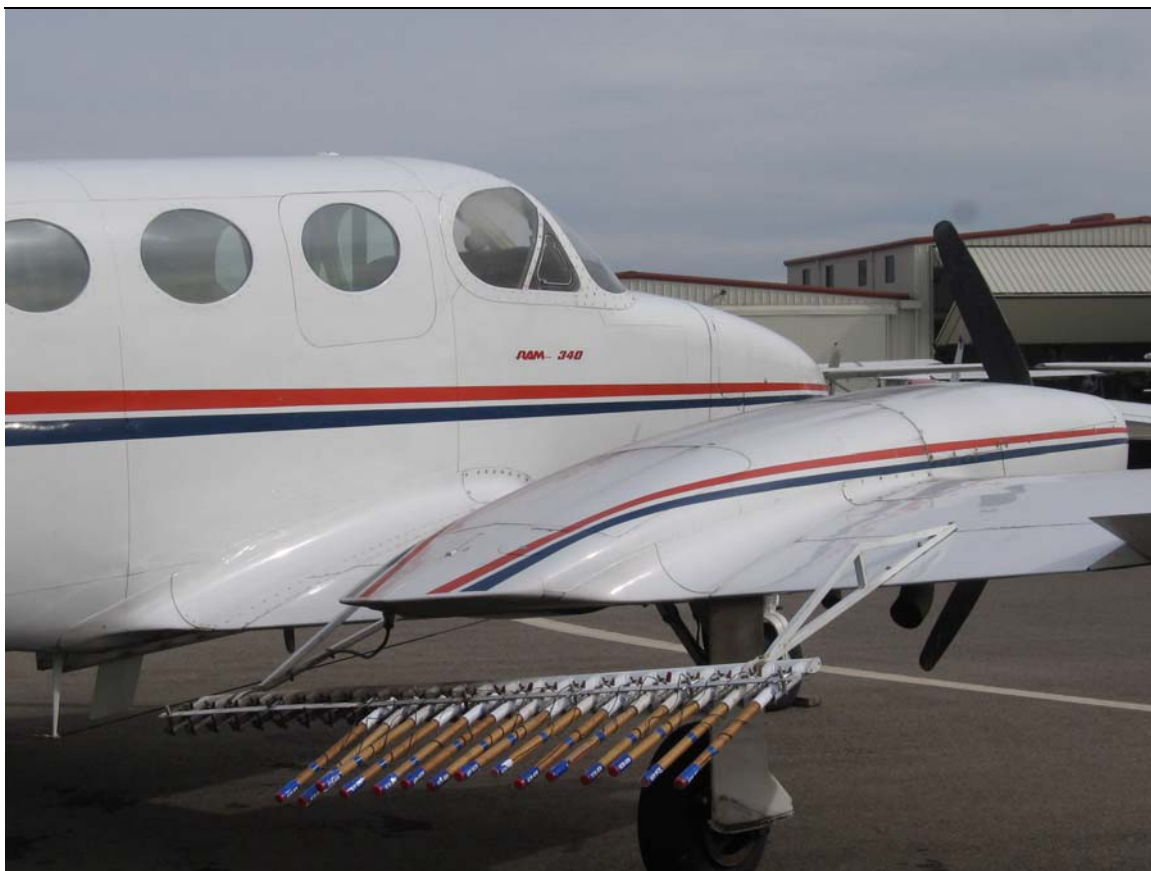
Figure 3.6 Aircraft with Seeding Flare Racks
