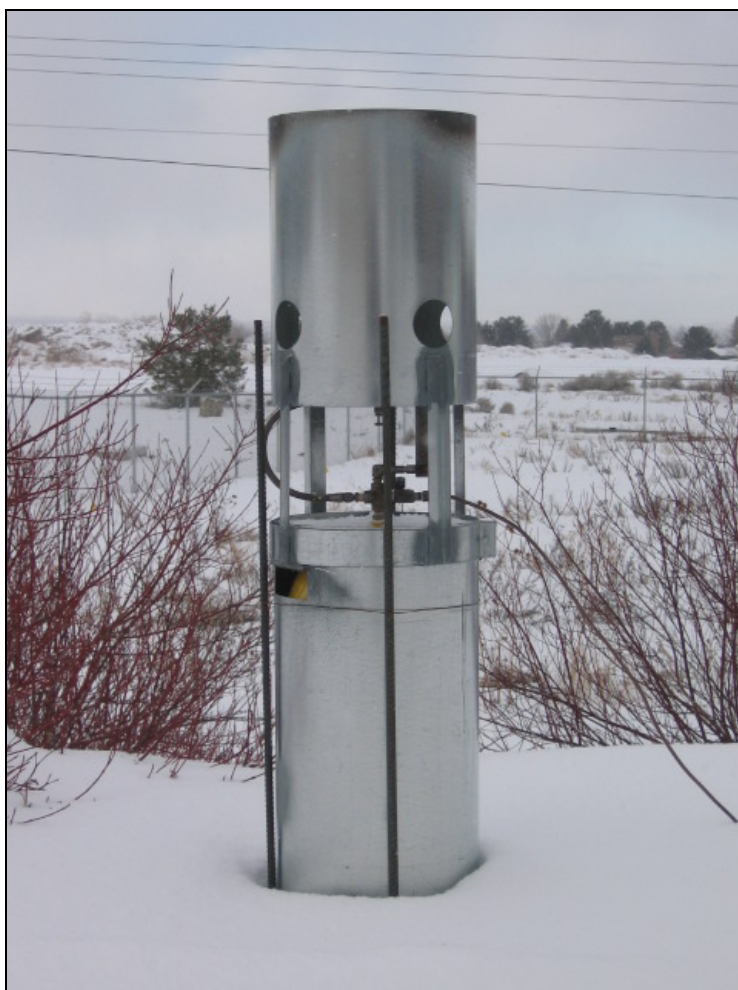
Figure 5.2 Cloud Nuclei Generator (CNG)
