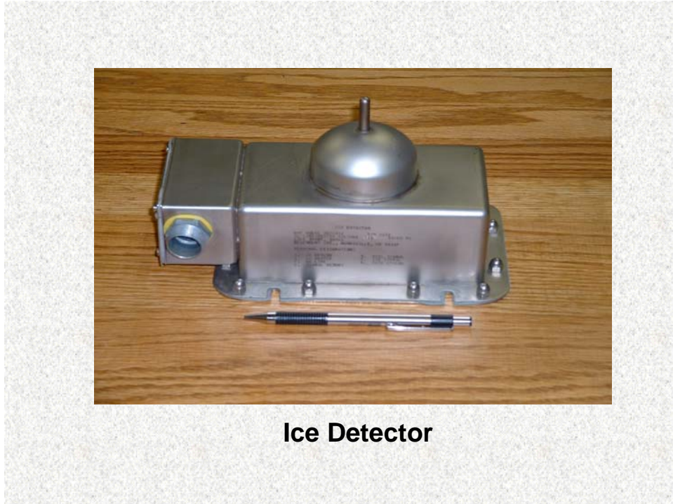
Figure 8.1 Icing Rate Meter
