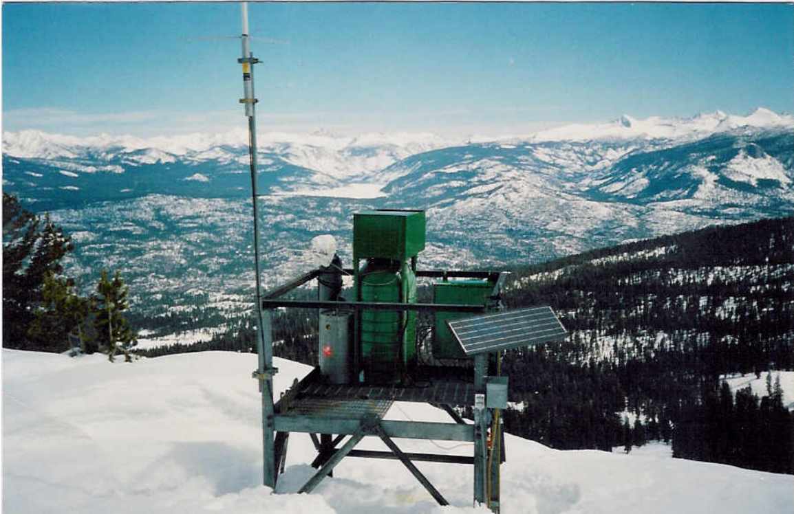
Figure 3.3 Remotely Controlled, Ground-based Silver Iodide Generator
