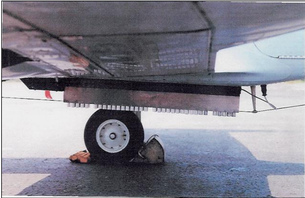
Figure 3.9 Aircraft Belly Mount, Droppable Silver Iodide Seeding Flare Rack
