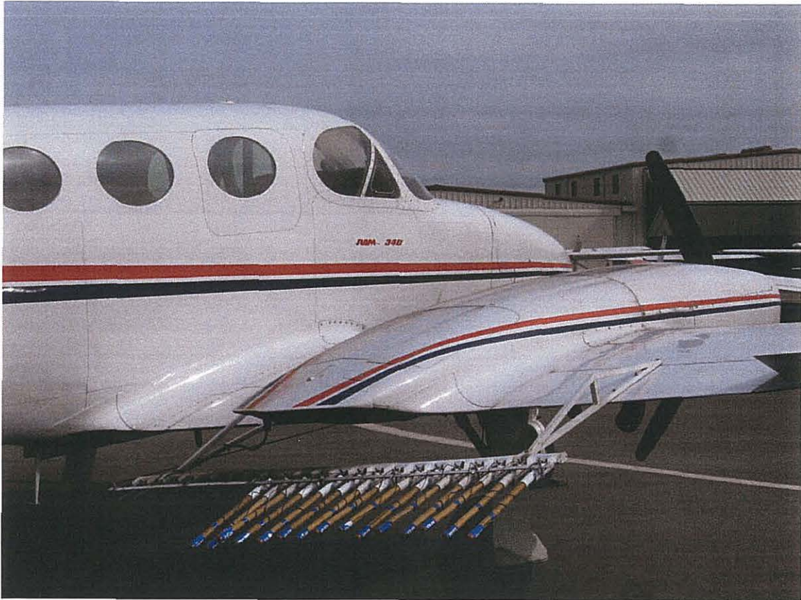
Figure 5.9 Aircraft with Seeding Flare Racks
