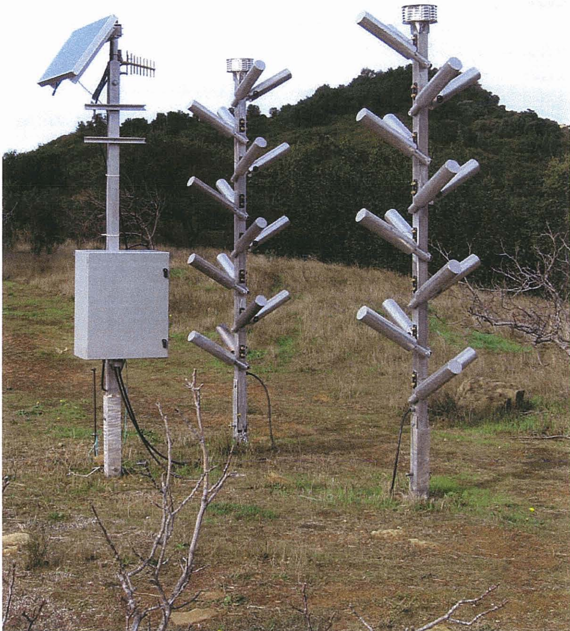
Figure 5.8 Ground-Based Seeding Flare Site
