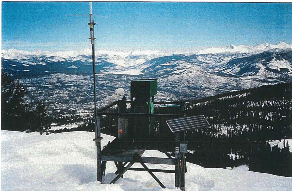
Figure 5.6 Remotely Controlled, Ground Based Silver Iodide Generator
