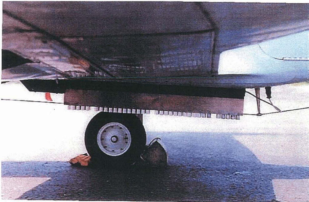
Figure 5.12 Aircraft Belly Mount, Droppable Silver Iodide Seeding Flare Rack
