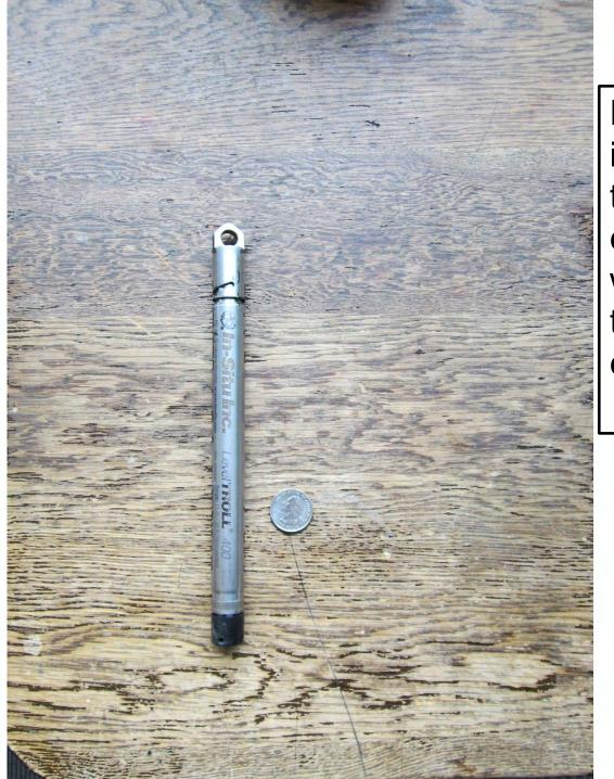
In 2012, IDWR began installing pressure transducers in wells for continuous ground water level and water temperature data collections.
