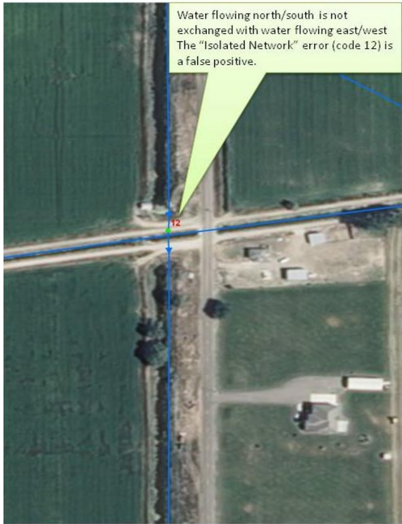
Figure 8 - Example of flume/siphon location at the intersection - over/under segments.
