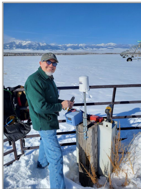
Tito Sanabria, IDWR's telemetry expert, installs telemetry at a data collection station in Salmon, Idaho. Image courtesy of Tito Sanabria, IDWR.
