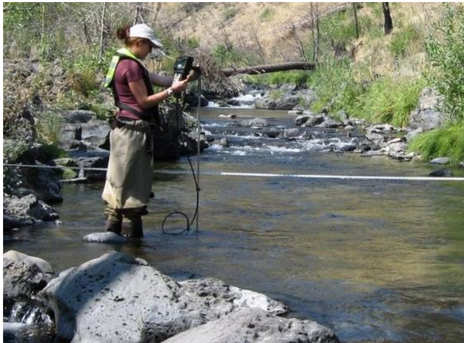
Figure 4. A USGS hydrologist using an ADV device (FlowTracker) to make a direct velocity flow measurement across a transect.
