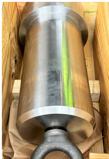
Above left, new trunnion pin ready for installation. Right, workers install a pin and bushing assembly on a spillway gate. (photos courtesy Bureau of Reclamation)
