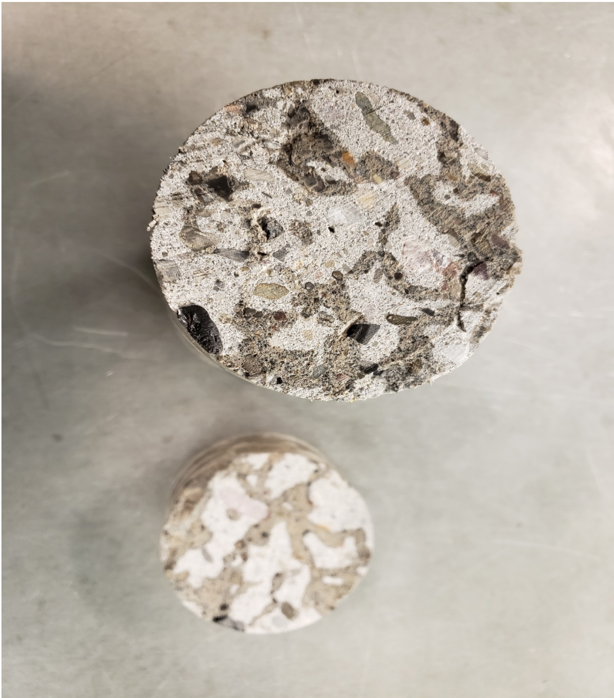
Moisture throughout Core #5 After being Cut
