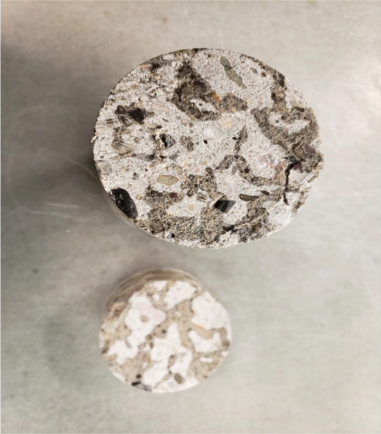
Moisture throughout Core #5 After being Cut
