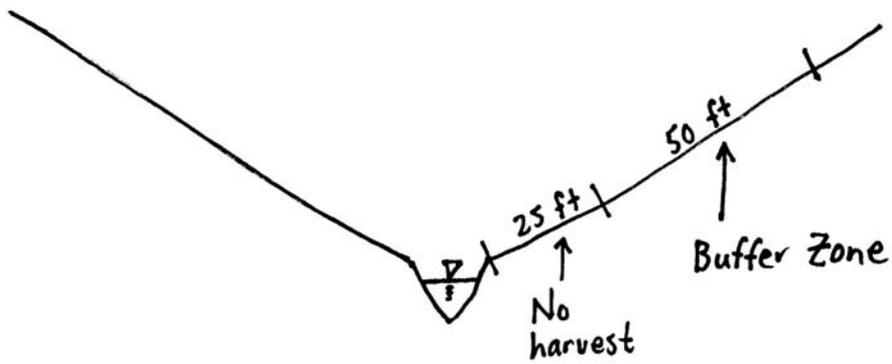
Figure 2. Stream is stable in an un-confined valley.
