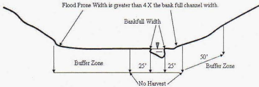
**SINGLE UNCONFINED CHANNEL:** Bank full flow is contained within a single channel and the flood prone width is greater than four times the bank full channel width.
