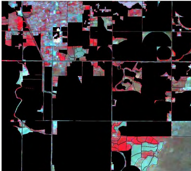
Figure 6. Irrigated polygons masked to black and superimposed on Landsat data from May 19, 2006.
