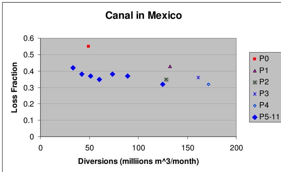
Figure 10. Mexico canal loss fractions (see Contor, 2004)
