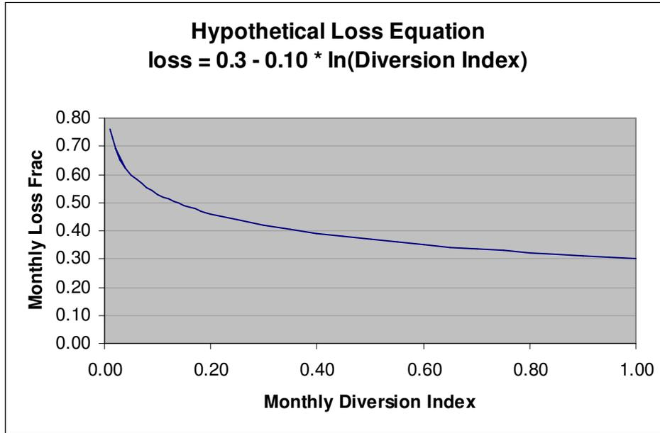
Figure 11. Graphical representation of equation (2).
