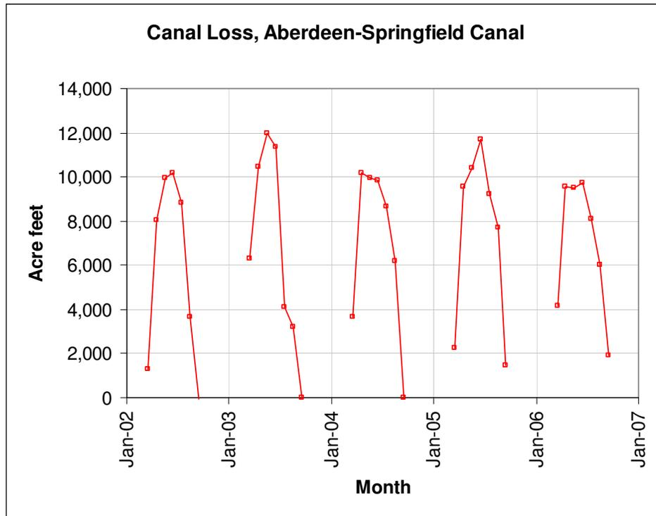
Figure 3. Canal loss of Aberdeen-Springfield Canal, volume per month, 2002 through 2007<sup>4</sup>
