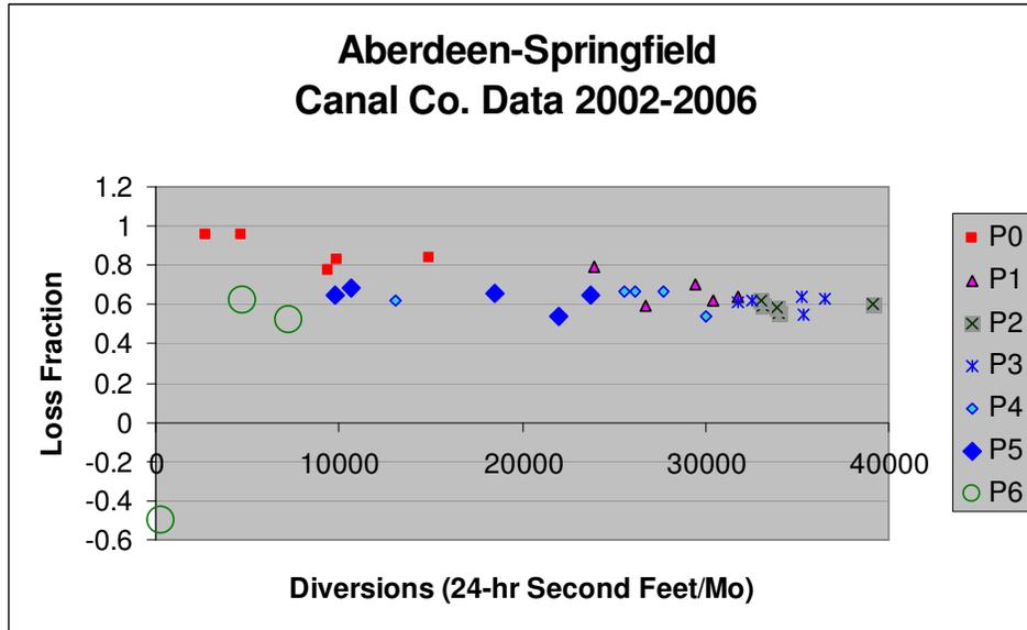
Figure 9. Aberdeen-Springfield Canal loss fractions (Data courtesy Howser, 2007)
