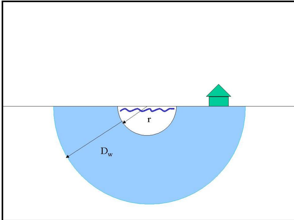
Figure 1. Hypothetical wetted bulb beneath a canal.
